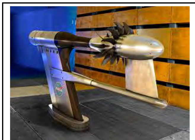
NASA research on future aircraft engine designs, such as the “Open Rotor”, aims to reduce the environmental impact of aviation.
