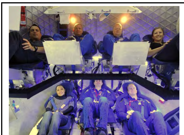
Crew system engineers and NASA astronauts evaluate the layout of the Dragon crew capsule on the factory floor at the Space Exploration Technologies (SpaceX) facility in Hawthorne, California. The new spacecraft is based on the Dragon cargo vehicle that successfully demonstrated its capability to carry cargo and experiments to and from the International Space Station.
