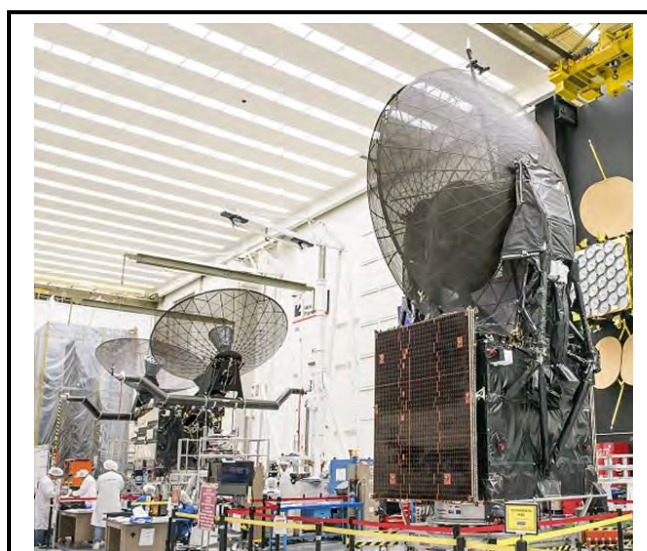
Antennas furled and solar panels folded, TDRS-K stands ready to package and ship to Florida for launch in early 2013. Its twin, TDRS-L, is undergoing preflight testing and will launch early in 2014. These spacecraft along with TDRS-M, which is in fabrication, will relay science data and commands to and from NASA customer missions like the ISS, Hubble, and Terra, as well as future missions like Orion Multi-Purpose Crew Vehicle and commercial crew spacecraft.
