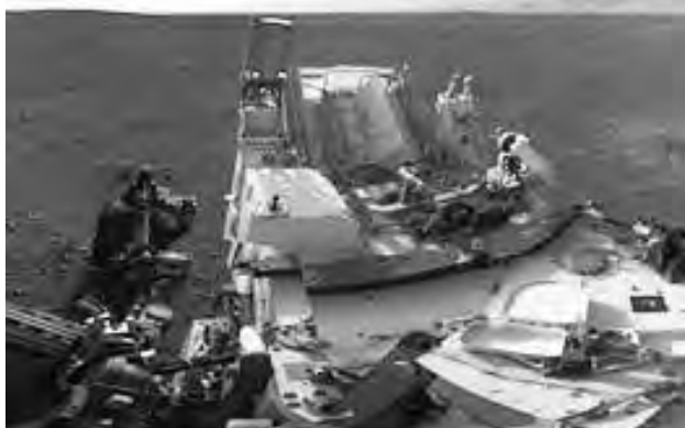
Curiosity took this self-portrait which shows its Multi-Mission Radioisotope Thermoelectric Generator or MMRTG, essentially a nuclear battery that reliably converts heat from the natural decay of the radioisotope into electricity. Instead of the solar panels used on Spirit and Opportunity, this power source was selected to provide greater mission flexibility in accessing difficult or remote terrain and enable continuous operation in the dusty Martian environment and throughout its winter season. The heat is also distributed internally to maintain effective operating temperatures for its instruments and systems.
