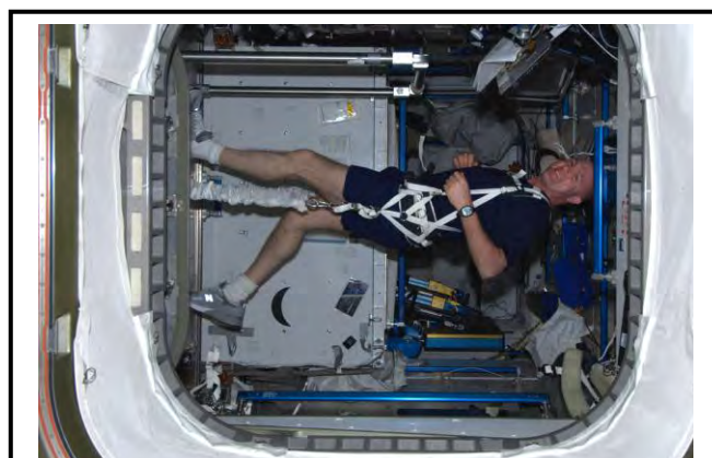
European Space Agency astronaut André Kuipers (ESA), Expedition 30/31 flight engineer, exercises using the advanced resistive exercise device (ARED) aboard the International Space Station. This apparatus has distinct advantages over previous space exercise machines in that it allows for more consistent load bearing and a wider range of movements. The Human Research Program recently published results demonstrating that current crew exercise prescriptions using the ARED combined with appropriate nutrition is an effective countermeasure against bone and muscle loss.
