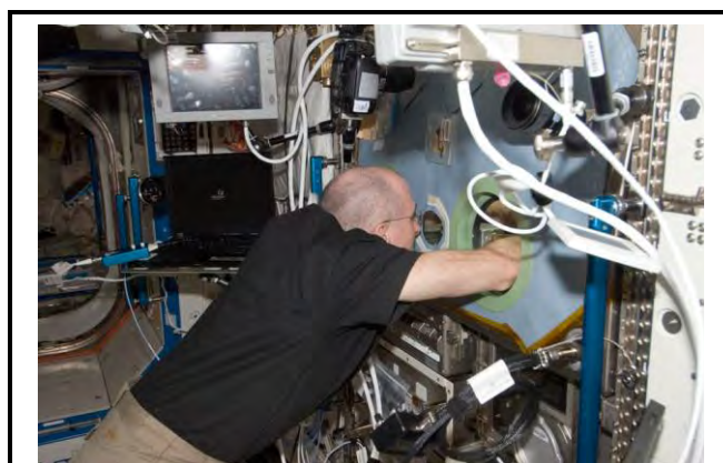
Don Pettit, ISS Expedition 30 flight engineer, works with colloidal particles in the microgravity sciences glovebox in March of 2012, studying interactions between particle surfaces and solvents. Results of this experiment will enable scientists to create models and processes to better preserve food and chemicals, evenly distribute ingredients to produce glues, jellies and gelatins, and control light movement in optical devices and materials.
