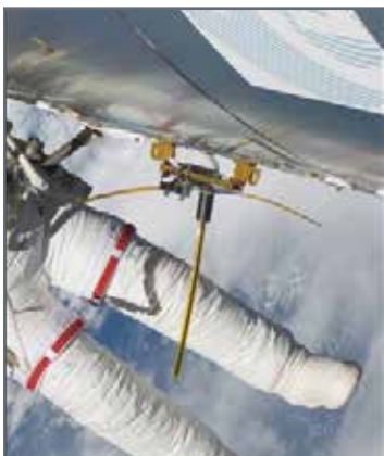
VIS Antenna shown installed on the external surface of the Columbus module.
