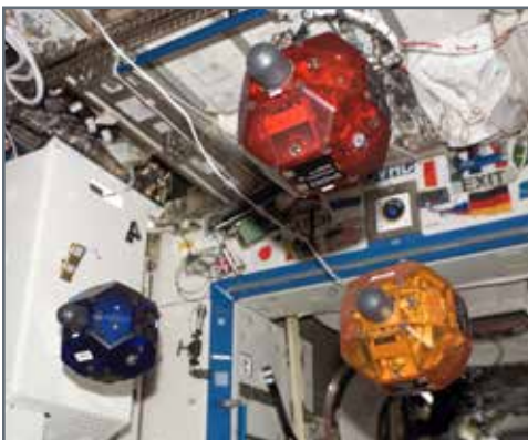
NASA Image ISS017E017377 - Above, Astronaut Greg Chamitoff, Expedition 17, programs the SPHERES satellites to perform a coordinated flight task.
