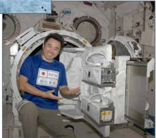
NASA Image: iss033e006452 - Astronaut Akihiko Hoshide posing with J-SSOD before it enters the JEM airlock for its initial CubeSat deployment operations during Expedition 32.
