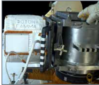
Image © Roscosmos: URM-D multipurpose workstation with integrated Photon-Gamma experiment taken during Increment 26 EVA-28.
