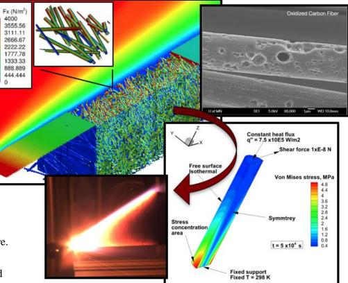
Molecular simulations of boundary layer flow at relevant hypersonic conditions (top-left) will provide the local chemical environment and structural loading for microstructure features. Microscale modeling of coupled chemical (top-right) and structural (bottom-right) response will enable prediction of spallation (bottom left) as well as computational design of TPS at the microstructure level.
