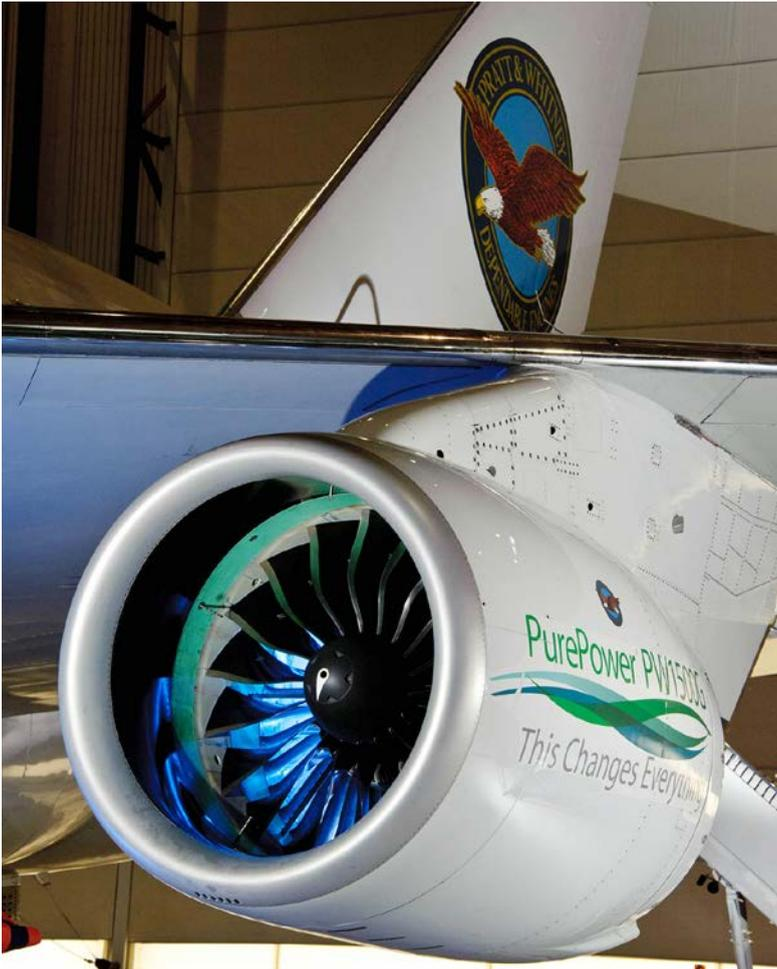
**Figure 7-3.** Pratt & Whitney's Geared TurboFan technology became the basis for the PurePower engine series. (Pratt & Whitney)
