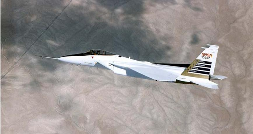
Dryden researchers used a NASA F-15 to test the Digital Electronic Engine Control (DEEC) system from 1981 to 1983. (NASA)
