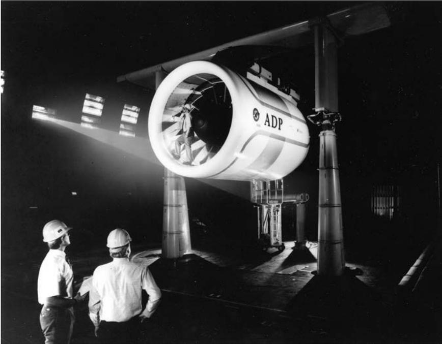
**Figure 6-4.** The Pratt & Whitney and NASA team prepare the Advanced Ducted Propulsor (ADP) for a flow visualization test in the National Full-Scale Aerodynamics Complex (NFAC) 40- by 80-foot Wind Tunnel at the Ames Research Center. (NASA)
