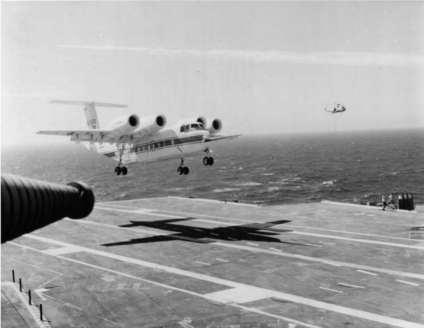
**Figure 3-3.** The QSRA made over a dozen landings on the U.S.S. *Kitty Hawk* during naval flight trials near San Diego, CA, in August 1980. (NASA)
