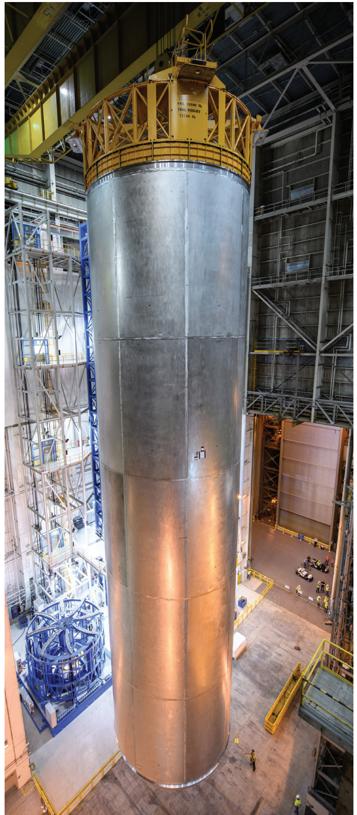
A qualification test article for the liquid hydrogen tank on NASA's new heavy-lift rocket, the Space Launch System, is lifted off Michoud's Vertical Assembly Center after final welding is complete. (NASA/MSFC/MAF)
