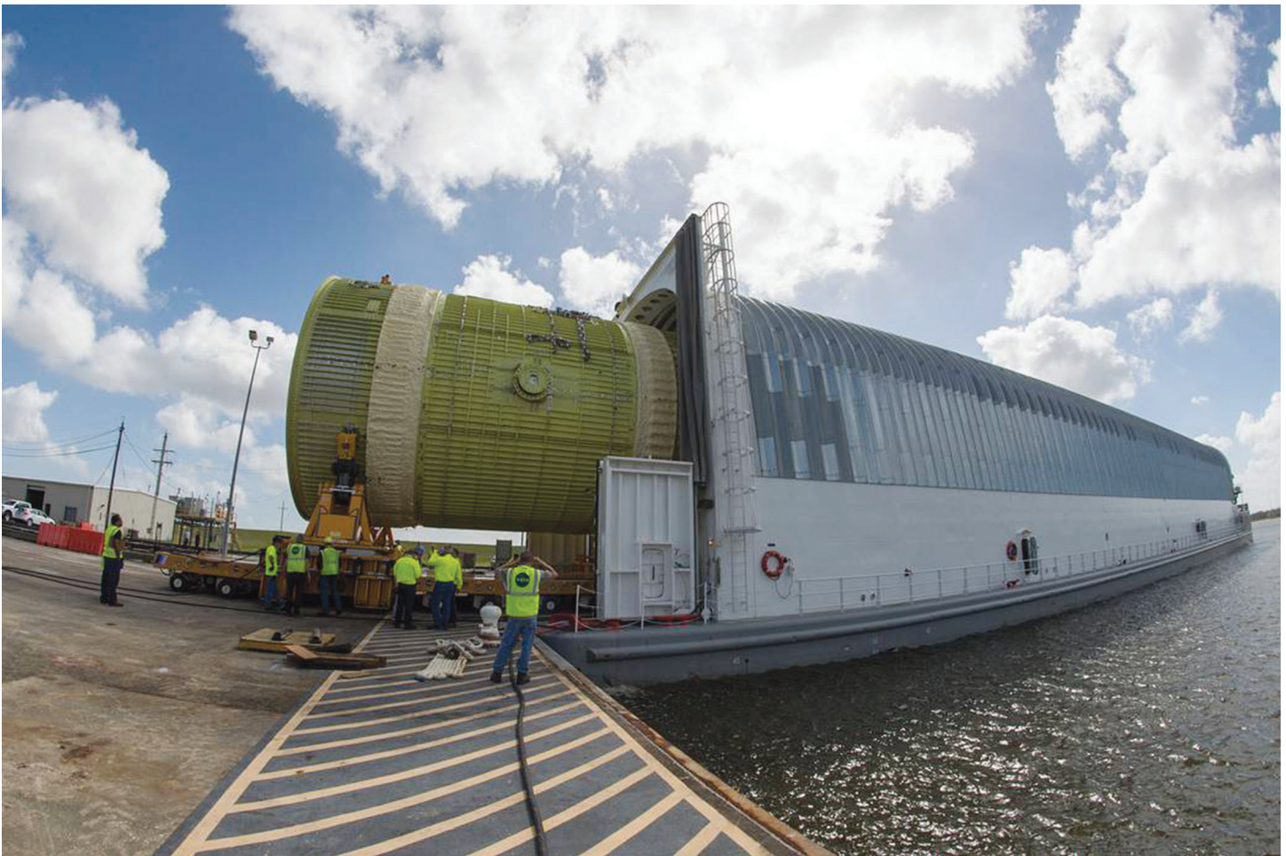
A structural test version of the intertank for NASA's new heavy-lift rocket, the Space Launch System, is loaded onto the barge Pegasus, at NASA's Michoud Assembly Facility in New Orleans. Pegasus, originally used during the Space Shuttle Program, has been redesigned and extended to accommodate the SLS rocket's massive, 212-foot-long core stage — the backbone of the rocket.
