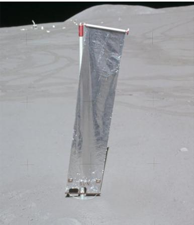
**Figure B9 – Solar Wind Composition Experiment
