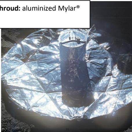
**Thermal shroud:** aluminized Mylar®
