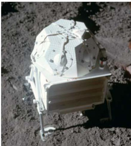
**Figure B5 – Solar Wind Spectrometer**
