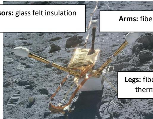
**Sensors:** glass felt insulation
