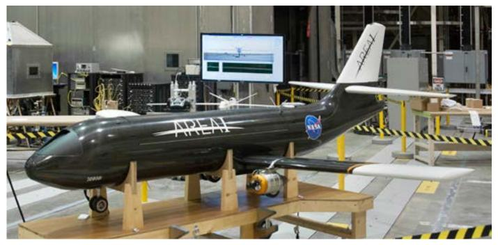
Seen here in the Armstong Flight Loads Laboratory, the semi-modular PTERA may be reconfigured to accommodate a wide variety of flight experiments. (NASA photo/Ken Ulbich
