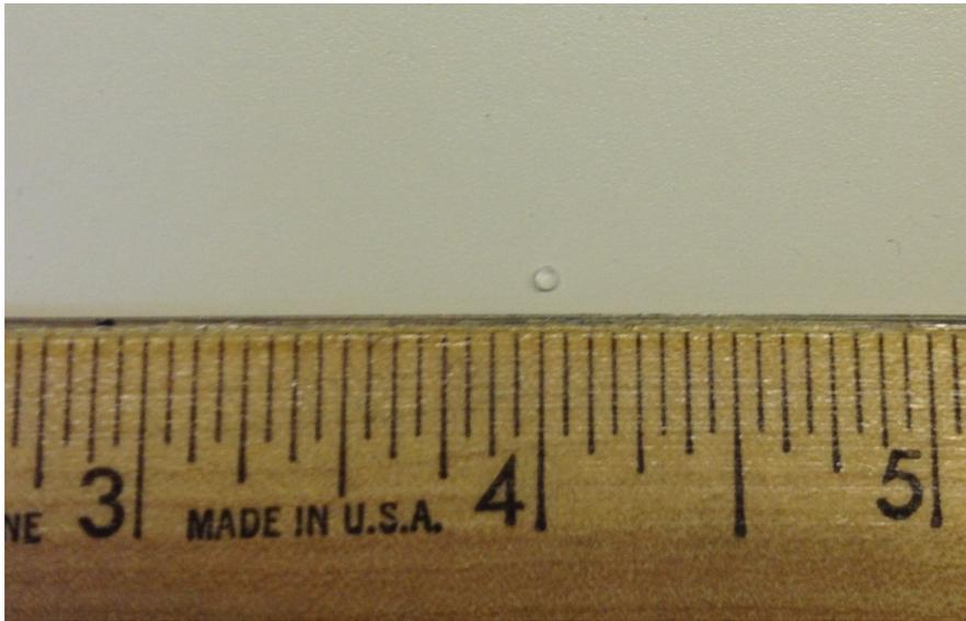
Figure 30. 0.3 mm hemispherical grain.
