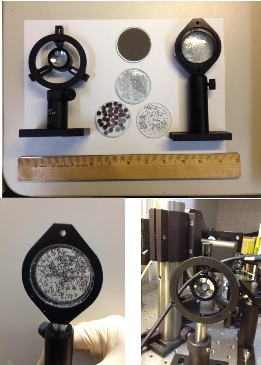
Figure 93. Different granular lenses used in the experiments.
