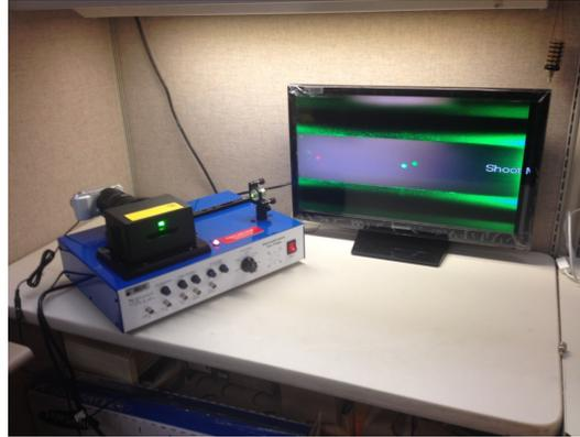
Figure 157. Installed ion trap set-up.
