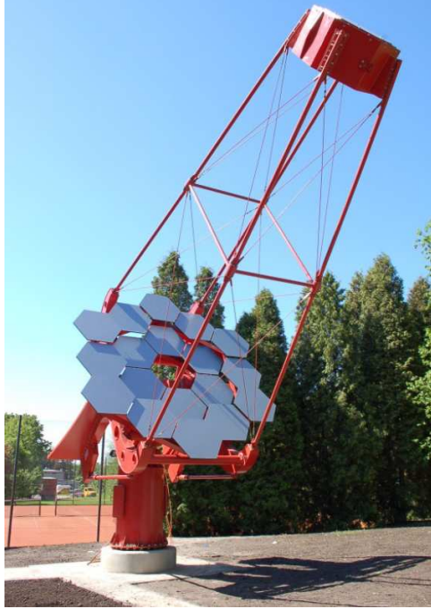
FIG. 9: An SST1M telescope is a workhorse of the CTA project. This telescope is designed for light collection rather than for imaging, which considerably offsets the costs of its mass-production.
