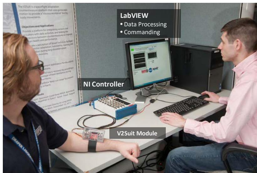
Figure 20 – V2Suit breadboard module worn and interfacing with a command and control computer.
