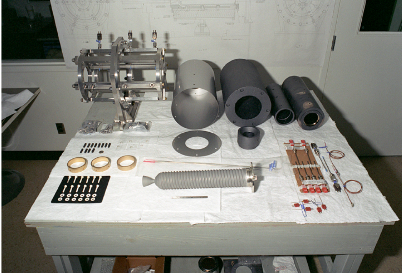
FIGURE 3.1. Components of the early Solar Thermal Propulsion Engine, presumably pre-Shooting Star Program. Courtesy of NASA MSFC.
