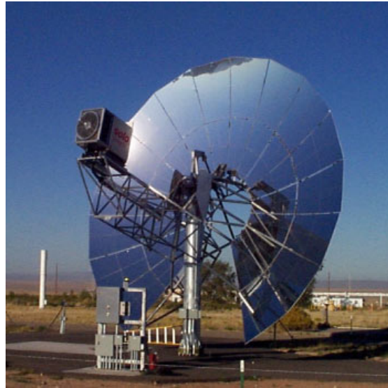
FIGURE 7.1. Parabolic Solar Concentrator focused on an electrical generator in the secondary reflector position.
