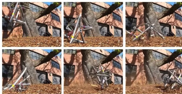
Figure 56: Drop test from 7.5m.
