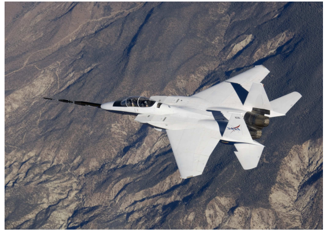
NASA Dryden Flight Research Center Photo Collection http://www.dfrc.nasa.gov/Gallery/Photo/index.html NASA Photo: ED06-0184-33 Date: September 27, 2006 Photo By: Carla Thomas NASA F-15B #836 in flight with Quiet Spike attached.
