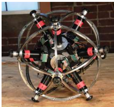
Figure 34: CMU RATS, a pneumatic hopping all-terrain robot
