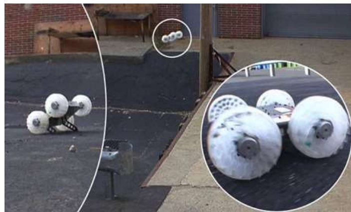
Figure 33: Combination driving and hopping robot: Boston Dynamics' Sand Flea.
