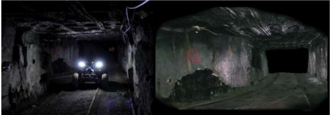
Figure 46: A mapping robot explores a terrestrial underground space using active illumination (left). An immersive virtual model of the environment is created using camera and LIDAR fusion techniques (right).
