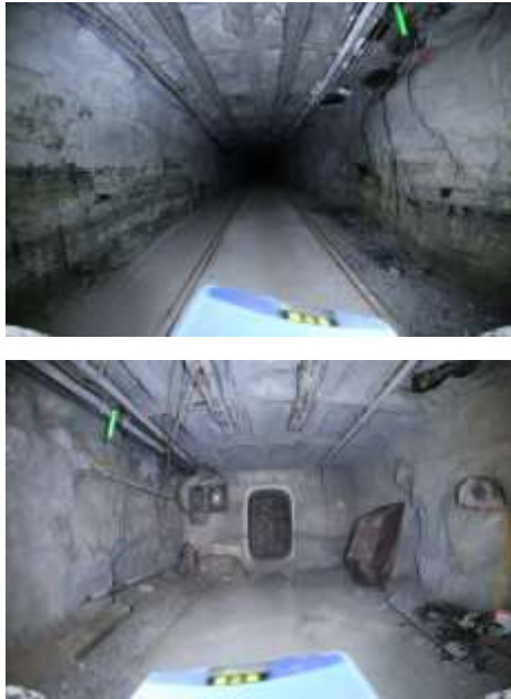
Figure 41: Concept for operation under reduced comm., showing difference between the cave exploring robot's high-definition view of the scene and the limited-data-rate model that the operator sees as the robot explores.
