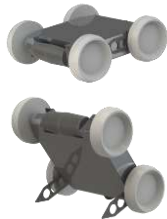
Figure 13: “Cavehopper”, a hybrid driving/hopping robot for planetary cave exploration.
