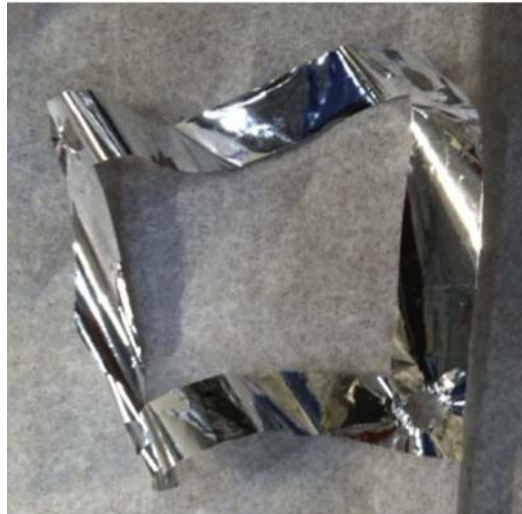
Figure 7.1: Warped membrane following ethanol sonic bath
