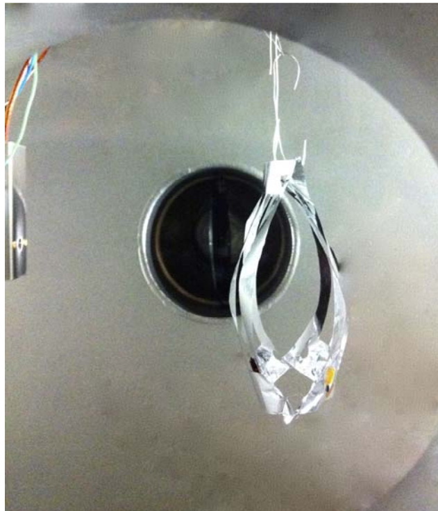
Figure 7.3: The \frac{1}{4} mil membrane structure inflated in the vacuum chamber
