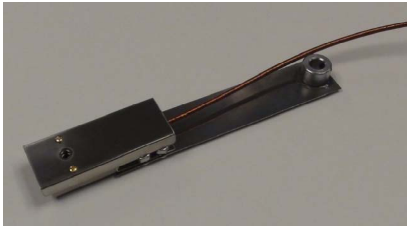
Figure 4.5 Mounted Faraday cup with collar for attachment to vacuum feedthrough
