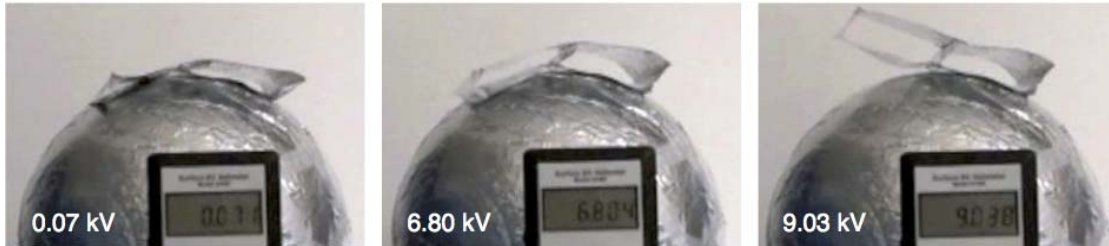
Figure 3.3: Atmospheric Electrostatic Inflation Experiment of a Box-Like Membrane Structure
