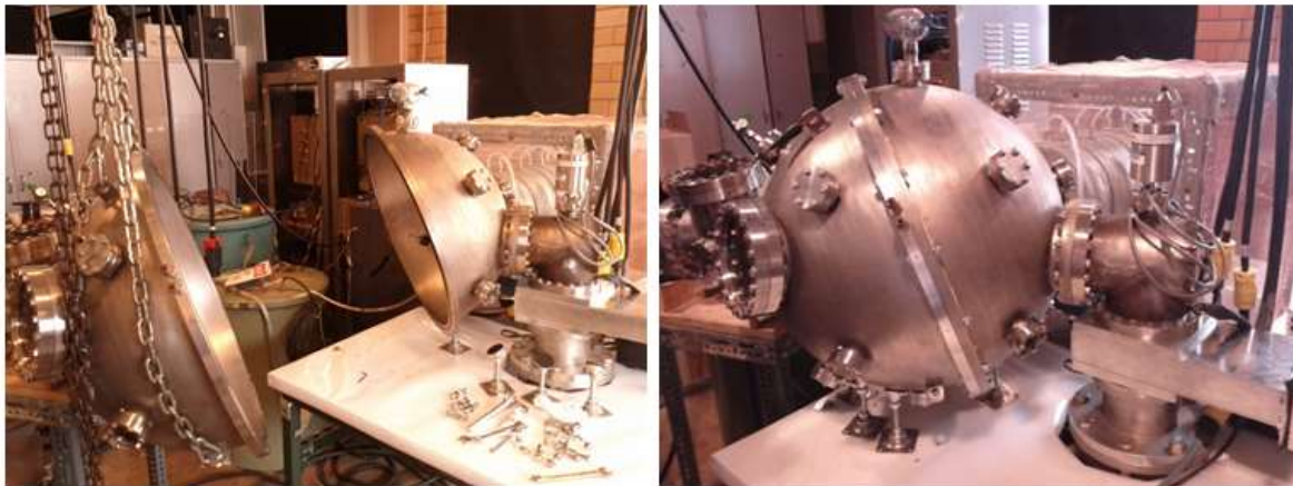
Figure 3.5.1-1. IEC Device at UIUC: 50 kV, 50 mA, 1 kW max. 44” diameter spherical stainless steel IEC chamber. Base vacuum <10^{-6} Torr.
