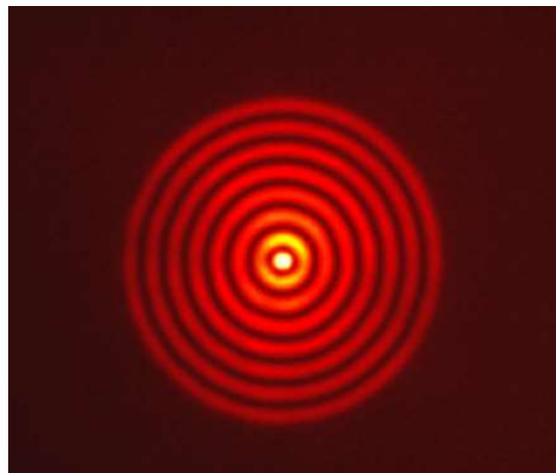
**Figure 5:** Transverse profile of Bessel beam.
