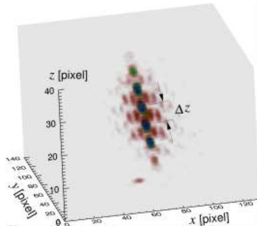
**Figure 6:** Volumetric reconstruction of an experimentally realized optical conveyor. This technology could trap multiple objects between each maxima.
