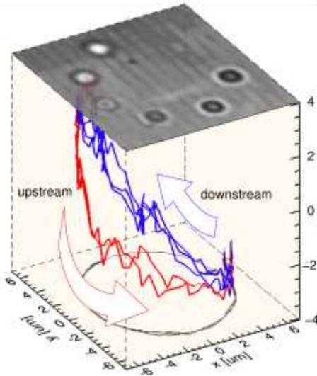
**Figure 5:** Experimentally measured trajectory of a colloidal silica sphere moving downstream (blue) and upstream (red) along a solenoid beam as the winding number is flipped from +30 to -30.
