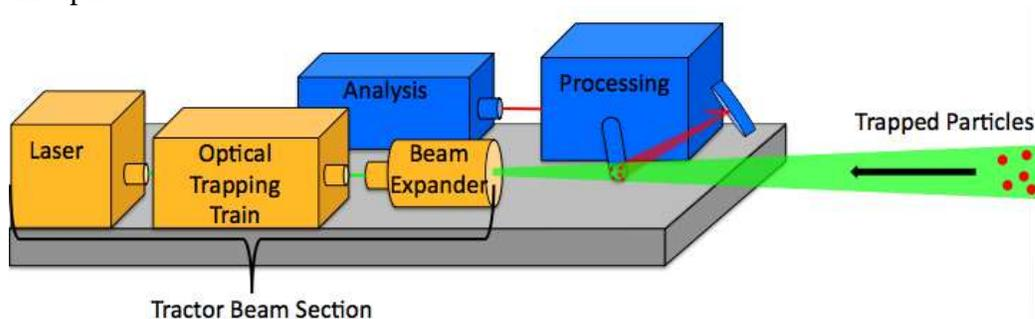
**Figure 11:** This is a systems view of the components that will need to be developed to make a full capture and analysis tractor beam instrument. The focus of this NIAC proposal will be to develop the yellow tractor beam system and eventually focus on coupling it to TRL 5+ processing and analysis devices.
