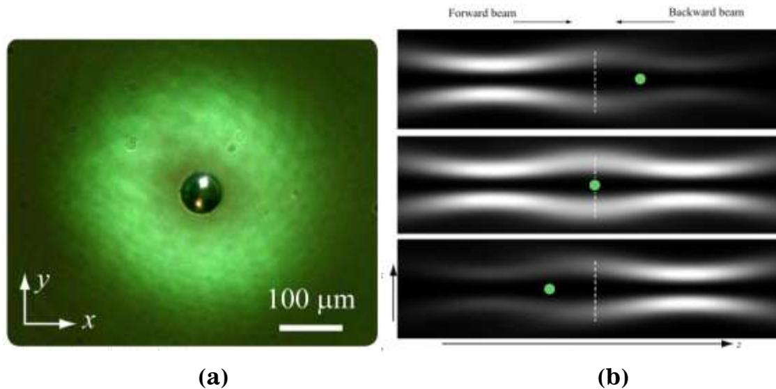
**Figure 8:** (a) Glass microsphere trapped in dark core of optical vortex, and (b) displacement of particle by variation of forward and backward beam intensities.
