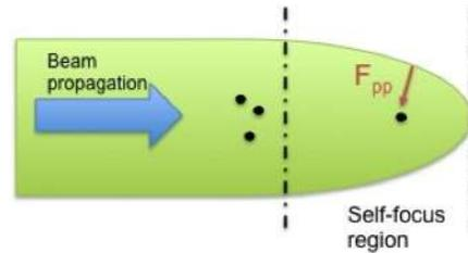
**Figure 5:** Particles in self-focused region of vortex beam experience force back along optic axis. Manipulation of the self-focusing effect could greatly increase the range of vortex traps.
