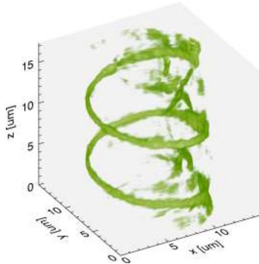
**Figure 4** Volumetric reconstruction of an experimentally projected optical solenoid beam, colored by intensity. The beam is propagating upward along  $z$ .
