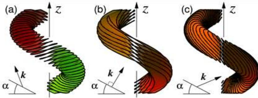
**Figure 3:** Controlling radiation pressure in a solenoid beam. (a) Wavefronts drawn as surfaces of constant phase direct radiation pressure downstream. (b) Radiation pressure is canceled by gradient forces when wavefronts are aligned with the spiral. (c) Retrograde tilt creates a solenoidal tractor beam.
