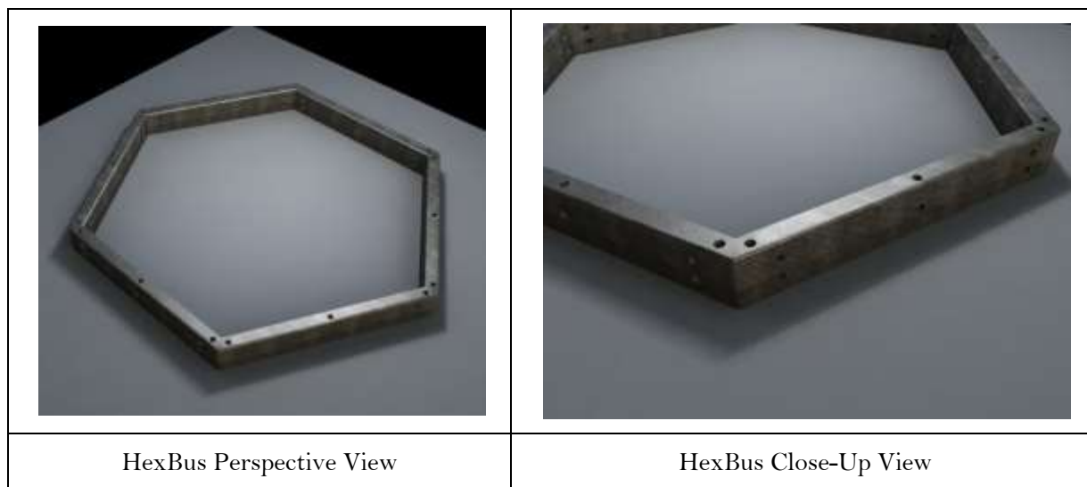
Figure 3-4 Illustrations of the “HexBus” Modular Spacecraft Concept
