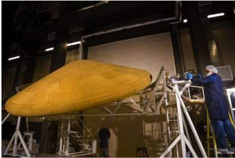
Figure 8: Mars Science Lab 4.5 m Diameter Heat Shield.
