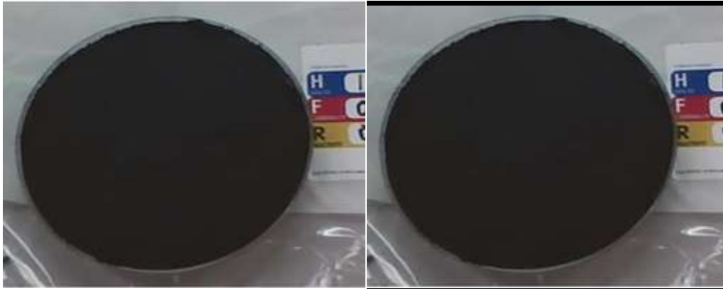
Figure 14. Initial RTV bound test tiles formed in a 3 inch diameter by ½” petri dish.
