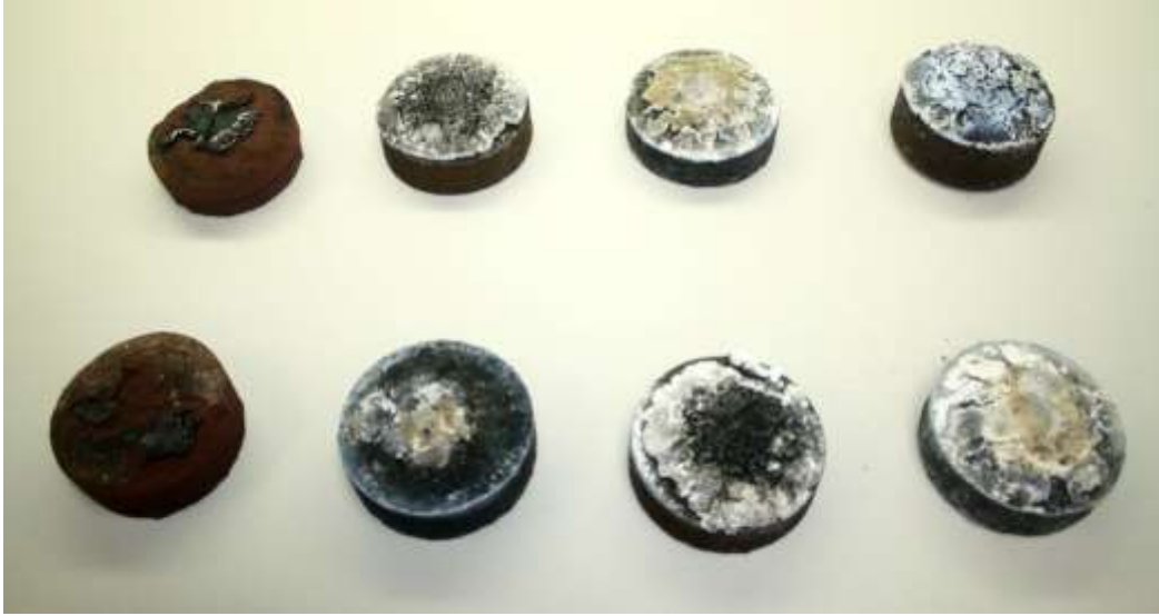
Figure 17. Post-test photo of the front surfaces of the eight flame test samples. The two JSC-1AC Lunar sintered samples are on the left-most column. The remaining samples on the top row are: RTV/JSC-1 Mars, RTV/JSC-1A Lunar, RTV/JSC-1 Mars. On the bottom row: RTV/JSC-1A Lunar, RTV/JSC-1 Mars, RTV/JSC-1A Lunar
