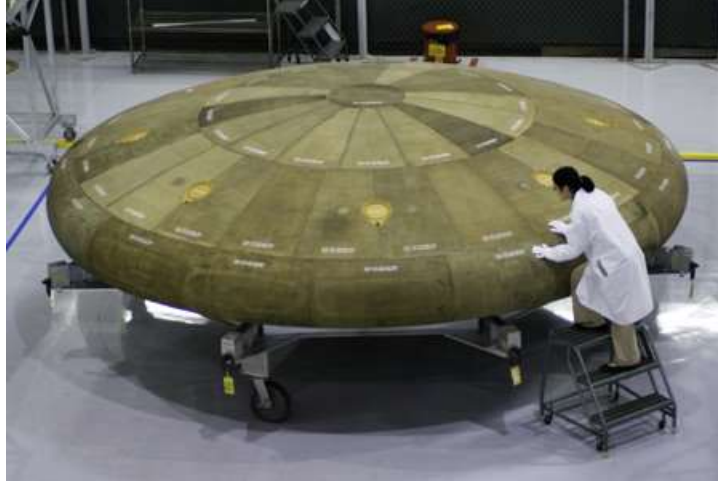
Figure 11: 5 m Diameter Ablator Heat Shield for NASA Orion Capsule.
