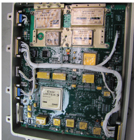
This image shows circuitry inside SpaceCube 2.0, which is flying on the military's STP-H4 instrument platform now operating on the International Space Station. This is the maiden voyage for SpaceCube 2.0, one in a family of advanced onboard processors.
