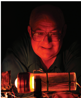
Principal Investigator Fred Minetto is bathed in a red glow produced by an electron gun, a key technology in a novel technique for cleaning mirrors and lenses. (Photo Credit: Pat Izzo)
