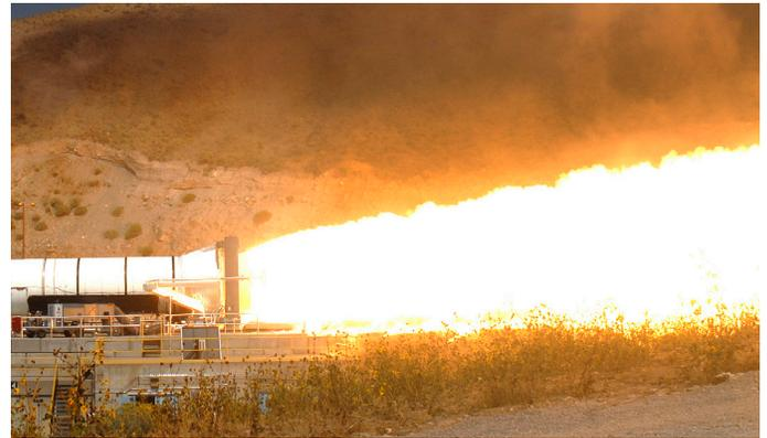
NASA and Orbital ATK have successfully completed four full-scale development test firings of the 5-segment solid rocket motor, as well as the important booster critical design review.
