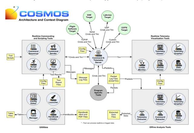
Figure 12.33: COSMOS architecture and context diagram. Credit: Ball Aerospace.
