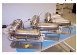
Figure 4.7: SSTL butane propulsion system. Credit: Surrey Satellite Technology Ltd.
