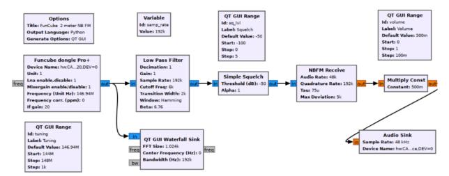
Figure 12.32: GNU Radio block diagram example for a 2-meter NBFM receiver. Credit: GNU Radio.
