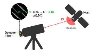
Figure 13.3: ELROI Optical Detection System. Credit: Los Alamos National Laboratory.
