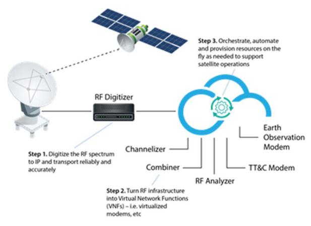
Figure 12.26: Kratos OpenSpace architecture concept. Credit: Kratos.
