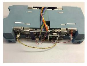
Figure 6.12: Illustration of the BioSentinel cold gas attitude control thruster. Credit: Lightsey et al. (2019).
