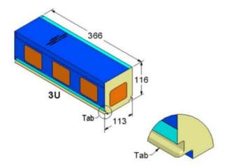
Figure 11.2: The Tab-type CubeSat. Credit: Planetary Systems Corporation.
