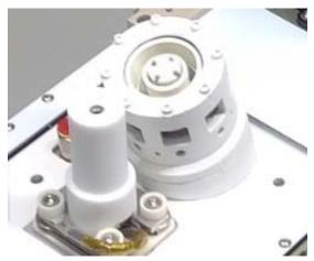
Figure 4.29: ExoMG-nano thruster. Credit: Exotrail.
