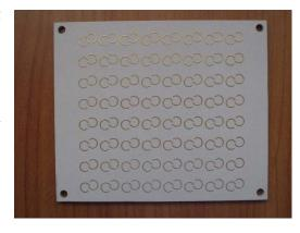
Figure 13.5: NTE Van Atta array retroreflector in the Ku-band, fits standard 1U panel, tuned to HAX RADAR frequency. Credit: Naval Information Warfare Center.
