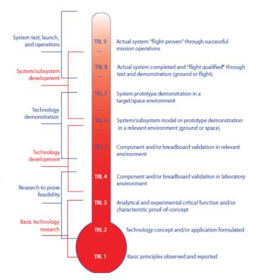
Figure 1.3: NASA's standard Technology Readiness Level (TRL) scale. Credit: NASA.
