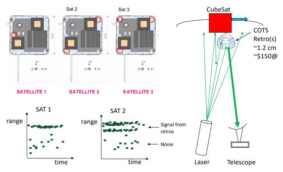
Figure 13.6: Corner Cube Reflectors. Credit: The Aerospace Corporation.
