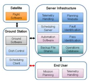
Figure 12.11: Software functions for elements within the ground segment. Credit: NASA.
