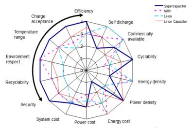
Figure 3.24: Supercapacitor comparison chart. Credit: Airbus Defense and Space and ESA (2016).
