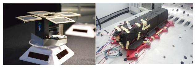
Figure 6.13: (left) Discovery 1P PocketQubes and (right) 3D printed AlbaPod 2.0 using Windform XT2.0. Credit: (left) Mini-Cubes and (right) Alba Orbital.
