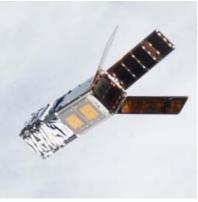
Figure 7.1: (top) Deployed Sunshield on CryoCube-1 and (bottom) CryoCube-1 in orbit with shield stowed. Credit: (top) Sierra Lobo and (bottom) NASA.
