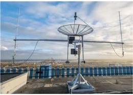
Figure 12.23: (left) ISIS ground station hardware, transceiver rack and (right) tracking antenna. Credit: ISIS.
