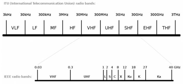
Figure 10.1: Radio spectrum used for spacecraft communication. Credit: NASA.
