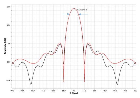
Figure 12.5: Antenna pattern from a 1.8 meter diameter parabolic dish operating at 915 Mhz with a high gain center lobe and diminished side lobes. Credit: NASA.
