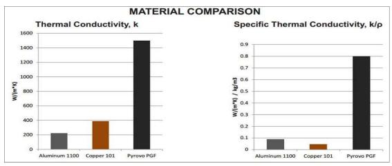
Figure 7.5: Pyrovo PGF Material Comparison. Credit: Thermotive Technology.
