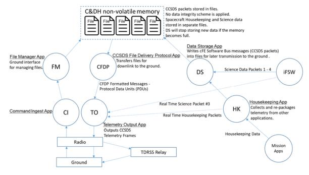
Figure 12.12: Command and telemetry data flow for a SmallSat mission using DTE and relay services. Credit: NASA.
