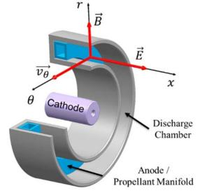
Figure 4.24: Hall-effect Thruster schematic. Credit: NASA.
