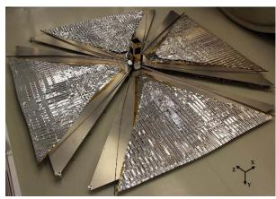
Figure 14.3: CanX-7 deployed drag sail during testing. Credit: Cotten et al. (2017).
