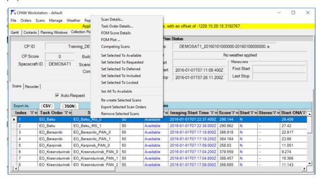
Figure 12.35: Orbit Logic CPAW couples spacecraft model and scheduling features to optimize data collection plans. Credit: Orbit Logic.
