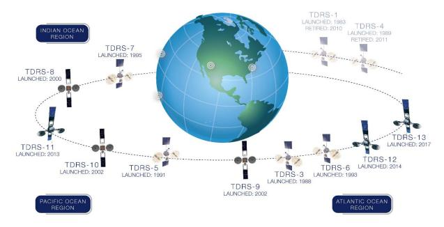
Figure 12.8: NASA's Tracking and Data Relay Satellite System. Credit: NASA.
