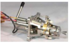
Figure 4.5: GR1 thruster. Credit: Aerojet.
