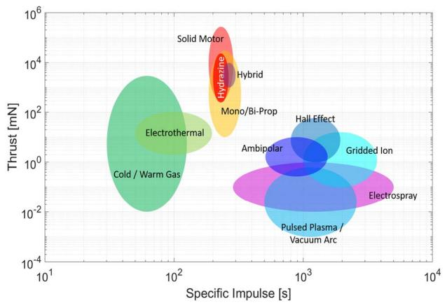
Figure 4.2: Typical small spacecraft in-space propulsion trade space (thrust vs. specific impulse). Credit: NASA.
