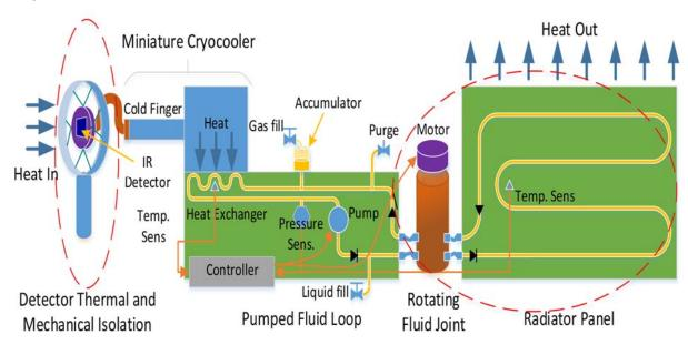
Figure 7.14: Conceptual operation of the ATA thermal control system. Credit: CSE/USU/NASA/JPL.
