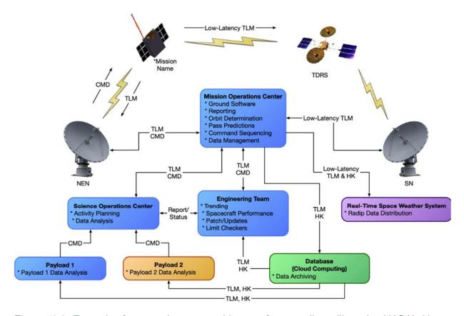
Figure 12.2: Example of a ground system architecture for a small satellite using NASA's Near Earth Network and Space Network. Credit: NASA.
