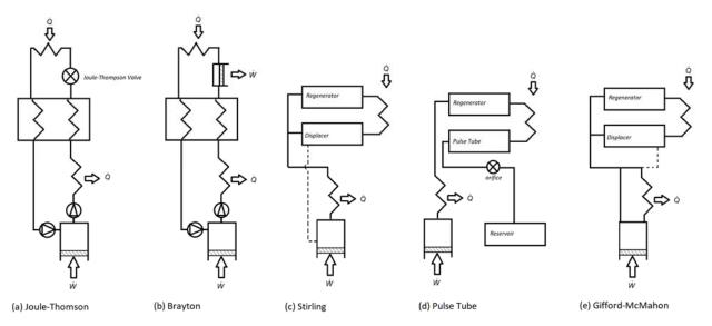
Figure 7.9: A comparison of cryocooler types. Credit: NASA.
