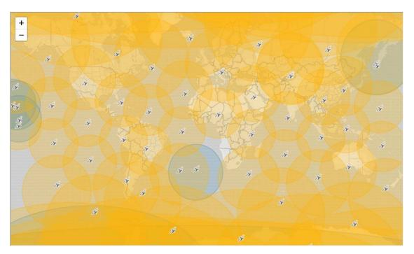
Figure 12.21 Screenshot of GSatTrack showing locations of Iridium Gen-1 satellites (blue circles) and Iridium NEXT satellites (orange circles). The size of the circle represents the coverage area. Credit: Global Satellite Engineering www.gsat.us.
