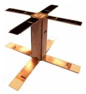
Figure 10.5: SNaP spacecraft with Haigh-Farr's deployable UHF Crossed Dipole antenna. Credit: Space Missile and Defense Command.
