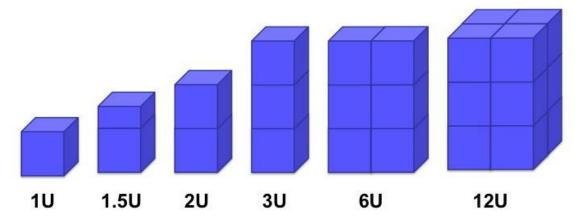
Figure 1.1: CubeSats are a class of nanosatellites that use a standard size and form factor. Credit: NASA.
