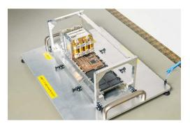
6.5: C3S *3U* CubeSat Structure. Credit: Complex Systems & Small Satellites.
