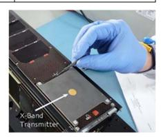
Figure 12.17: SeaHawk-1 CubeSat X-band antenna. Credit: NASA.
