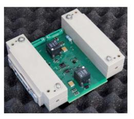
Figure 4.35: Plasma Brake Module (PBM) demo unit. Credit: Aurora Propulsion Technologies.
