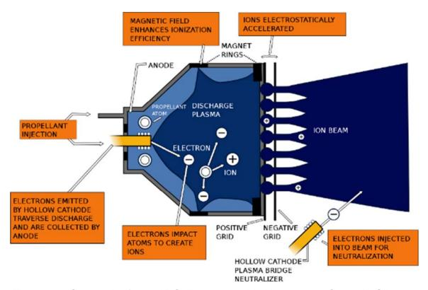
Figure 4.21: Schematic of typical DC-discharge gridded-ion thruster. Credit: NASA.
