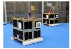
Figure 4.8: CanX-4 and CanX-5 formation flying nanosatellites with CNAPS propulsion systems. Credit: UTIAS SFL.
