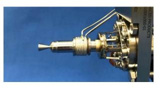
Figure 4.4: Plasma Processes LLC 100mN thruster. Credit: NASA MSFC.
