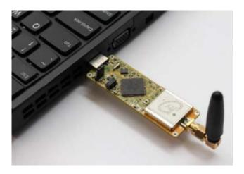
Figure 12.29: GAUSS UHF USB Mini Ground Dongle. Credit: GAUSS.
