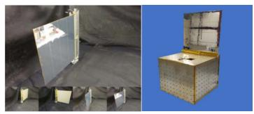
The design of a flexible deployable Figure 7.7: (left) 100W Deployable Radiator, and (right) radiator for small spacecraft was Radiator shown on ESPA structure. Credit: Thermal
