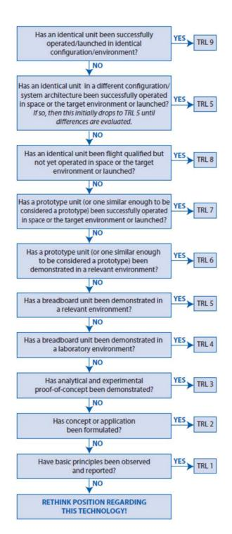
Figure 1.4: Technology Maturity Assessment (TMA) thought process. Credit: NASA.
