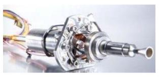
Figure 4.3: ECAPS HPGP thruster. Credit: Bradford ECAPS.
