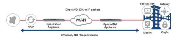
Figure 12.27: Kratos SpectraNet keeps most of the RF ground equipment remote from the ground station. Credit: Kratos.
