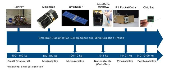
Figure 1.2: Overview of the variety of spacecraft that fall into the small spacecraft category. Credit: NASA and Adcole Space.
