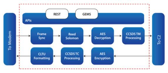
Figure 12.30: Kratos quantumFEP system architecture. Credit: Kratos.
