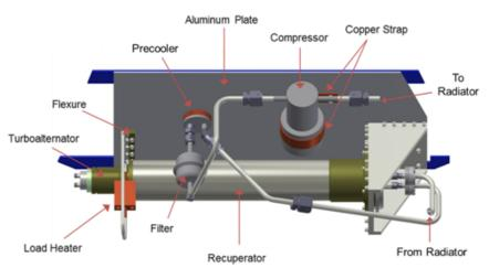
Figure 7.10: Configuration of primary mechanical UPL cryocooler components. Credit: Creare, Inc.
