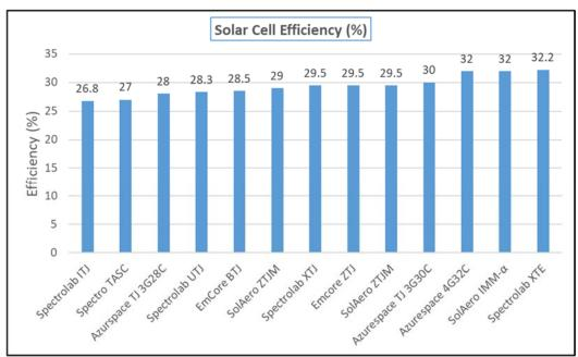
Figure 3.1: Solar cell efficiency. Credit: NASA.
