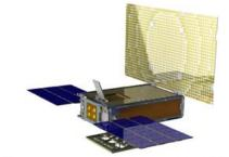
Figure 3.8: MMA's eHaWK solar array on the Mars Cube One (MarCO) CubeSat. Credit: NASA.
