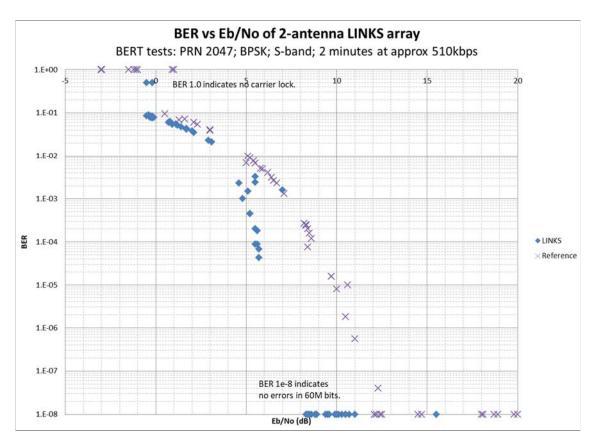
Figure 12.46: BER vs Eb/NO chart of ATLAS LINKS for S-band coded downlink. Credit: ATLAS Space Operations.
