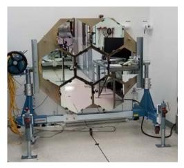
Figure 12.42: Prototype 7-segment mirror in lab testing at JPL. Credit: JPL.
