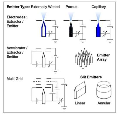
Figure 4.16: Schematic of typical electrospray emitter and electrode configurations. Credit: NASA.
