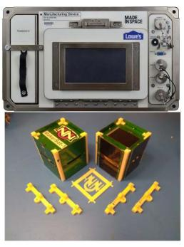
Figure 6.14: (top) Additive Manufacturing Facility onboard the ISS and (bottom) the MakerSat-1 CubeSat. Credit: Made in Space.
