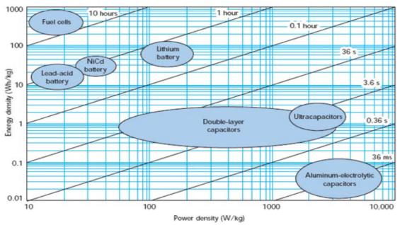
Figure 3.23: Relative power and energy densities Ragone chart illustration of different energy devices. Credit: US Defense Logistics Agency.
