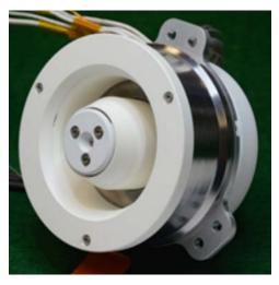
Figure 4.30: Halo thruster. Credit: ExoTerra Resource.
