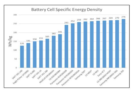
Figure 3.10: Battery cell energy density. Credit: NASA.
