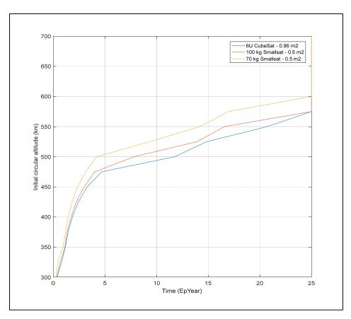
Figure 14.2: Initial orbit altitudes yield different lifetimes depending on the ballistic coefficient of the spacecraft. Three representative area-to-mass ratios are shown. Note that the propagation stops at 25 years, but the initial altitudes yield even longer times. Credit: NASA.
