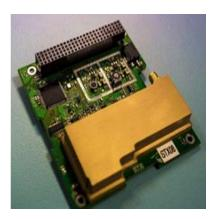
Figure 10.8: CubeSatcompatible S-band transmitter for either amateur or commercial bands. Credit: AAC Clyde Space.
