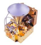
Figure 10.12: Ka-band transmitter with a horn antenna. Credit: Astro Digital.
