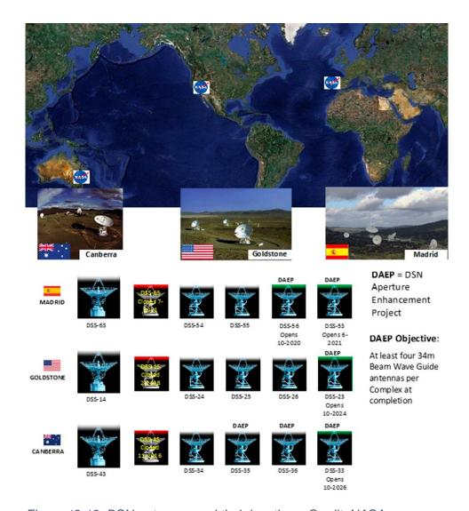
Figure 12.18: DSN antennas and their locations. Credit: NASA.
