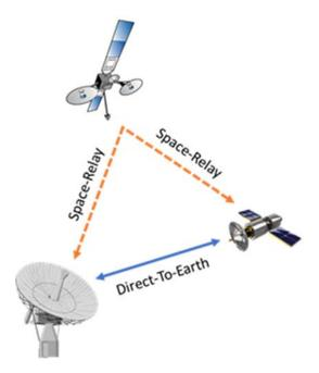
Figure 12.3: Illustration of Direct-to-Earth and Relay Concepts. Credit: NASA.
