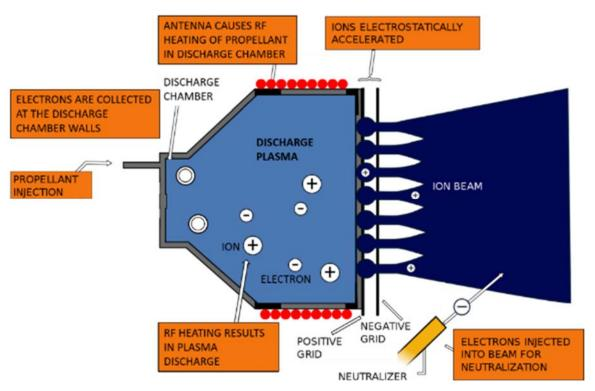
Figure 4.22: Schematic of typical RF-discharge gridded-ion thruster. Credit: NASA.
