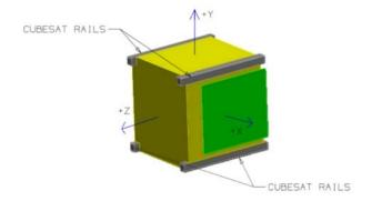
Figure 11.1: The Rail-type CubeSat. Credit: CalPoly's CubeSat Program.
