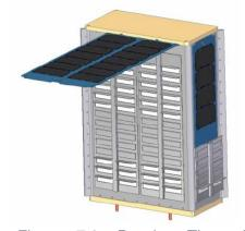
Figure 7.6: Passive Thermal Louver on 6U CubeSat Dellingr. Credit: NASA GSFC.
