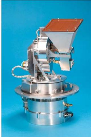
Figure 9.8. X-band high-gain antenna and pointing mechanism. Image courtesy of Surrey Space.
