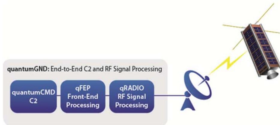
Figure 11.5. QuantumGND block diagram. Image courtesy of *RT Logic* (2015).
