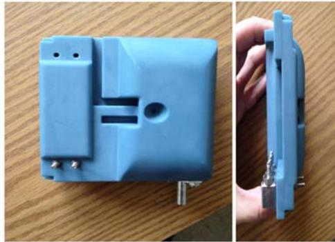
Figure 6.13. Cold Gas Propulsion Module fabricated using Accura Bluestone. Image courtesy of Steven Arestie, E. Glenn Lightsey, Brian Hudson (2012).
