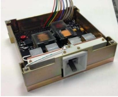
Figure 4.15. PPTCUP propulsion system. Image courtesy of Mars Space and Clyde Space Ciaralli et al. (2015).
