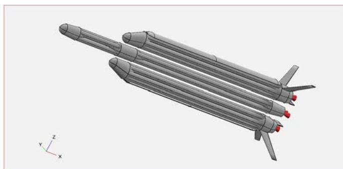
Figure 10.38. Austral Launch Vehicle Concept. Image courtesy of Heliq Advanced Engineering.
