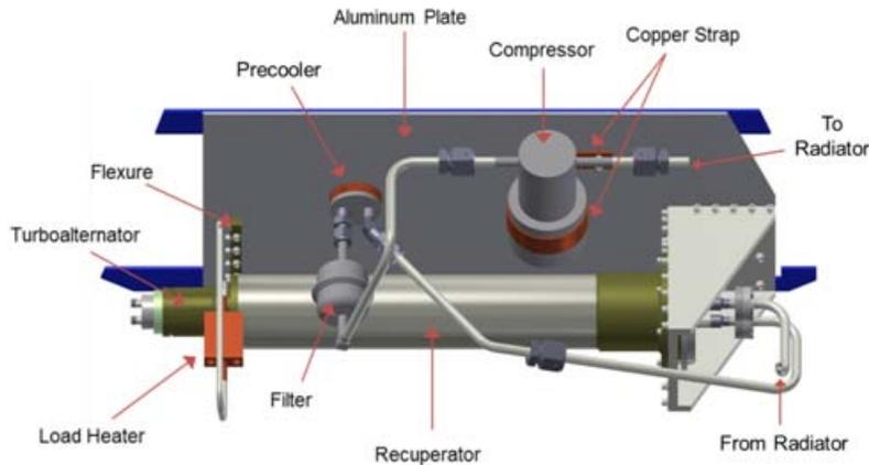
Figure 7.8. Configuration of primary mechanical UPL cryocooler components from Creare. Image courtesy of Zagarola et al. (2012).
