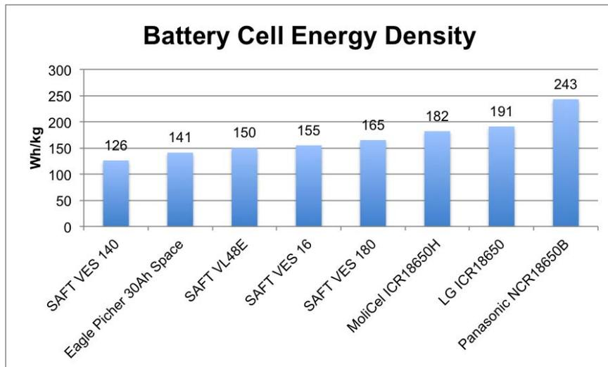
Figure 3.6. Battery Cell Energy Density
