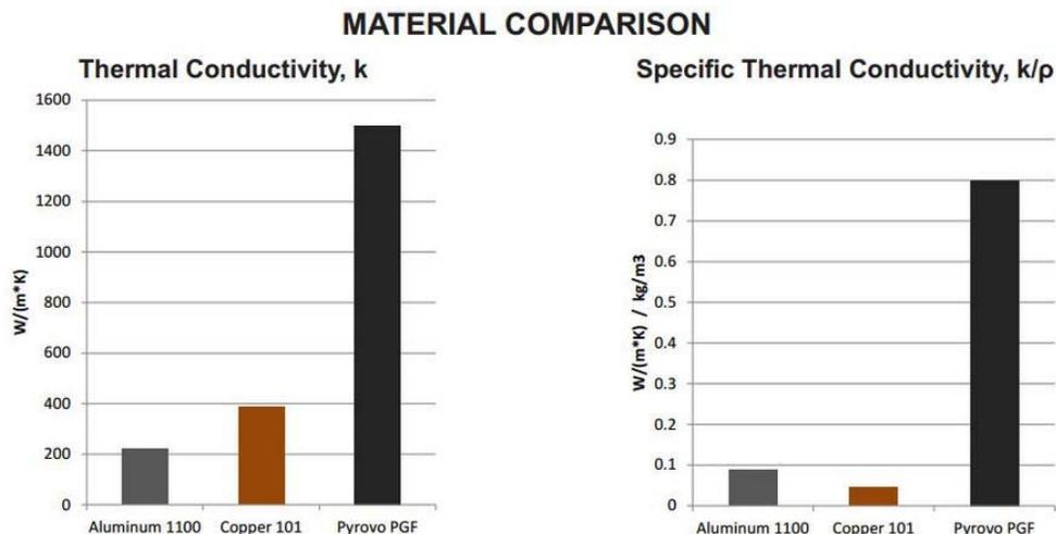
Figure 7.13. Thermotive Pyrovo PGF Material Comparison. Image courtesy of Thermotive (2014).
