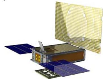
Figure 3.4. MMA's HAWK solar array on the Mars Cube One (MarCO) cubesat. Image courtesy of MMA (2015b).
