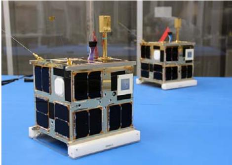
Figure 4.7. CNAPS spacecraft with UTIAS propulsion modules. Image courtesy of UTIAS website.
