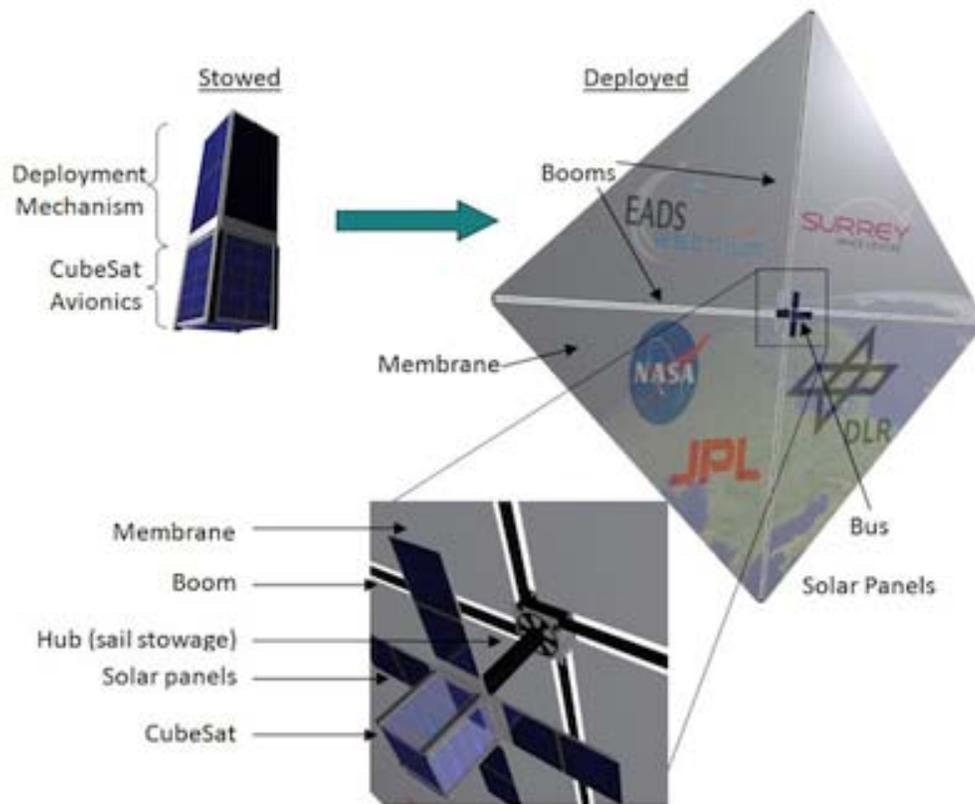
Figure 12.6. Labeled diagram of the Deorbital Sail concept. Image courtesy of University of Surrey (2015).
