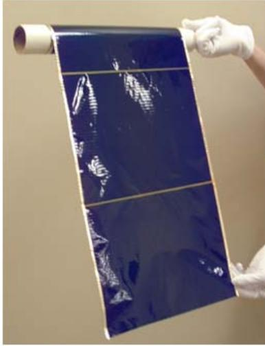
Figure 3.14. A series-connected string of production-sized cells on 1 mil polymer partially rolled onto a tube. Image courtesy of Casey (2014).
