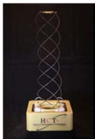
Figure 9.5. Example of deployable quadrifilar helical antenna. Image courtesy of Helical Communication Technologies.
