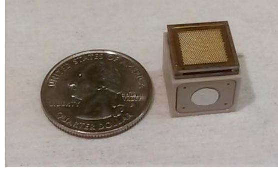
Figure 4.12. Electro spray thruster. Image courtesy of MIT SPL.
