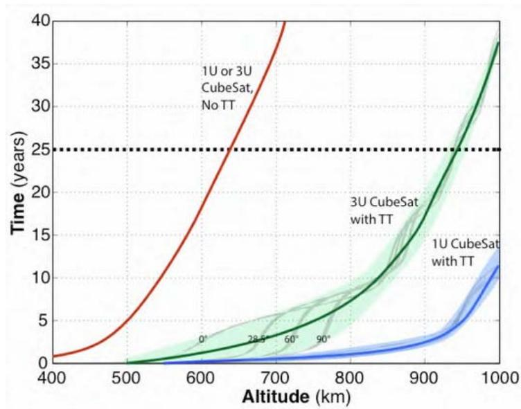
Figure 12.5. Performance curve of Terminator Tape for 1U cubesats in orbits up to 1200 km and for 3U cubesats up to 950 km. Image courtesy of Tethers Unlimited, Inc. (2014).
