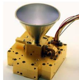
Figure 9.11. Ka-band transmitter with a horn antenna. Image courtesy of Aquila Space.
