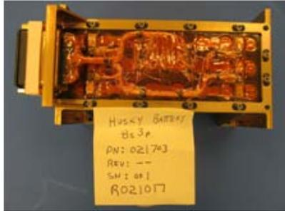
Figure 3.7. ABSL Commercial-off-the-shelf Li-ion Battery. Image courtesy of ABSL (2007).
