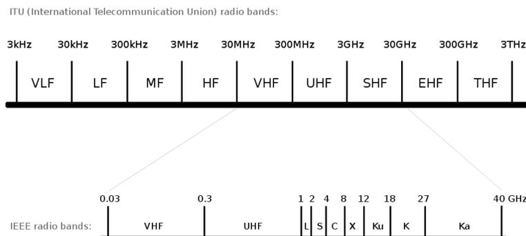
Figure 9.1. Radio spectrum used for spacecraft communication.
