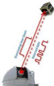
Figure 9.10. Scheme for using land based laser to transmit data from cubesat using on-board MRR. Image courtesy of Salas et al. (2012).
