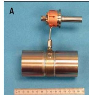
Figure 7.12. Flight design PT microcooler and its flight configuration with attached reservoir tank. Image courtesy of Durand et al. (2014).
