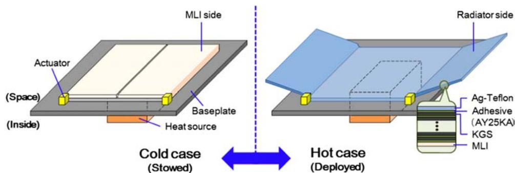
Figure 7.6. Flexible radiator conceptual diagram. Image courtesy of Ono et al. (2015).
