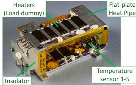
Figure 7.7. FOX flight model heat pipe developed at JAXA. Image courtesy of Nakamura et al. (2013).
