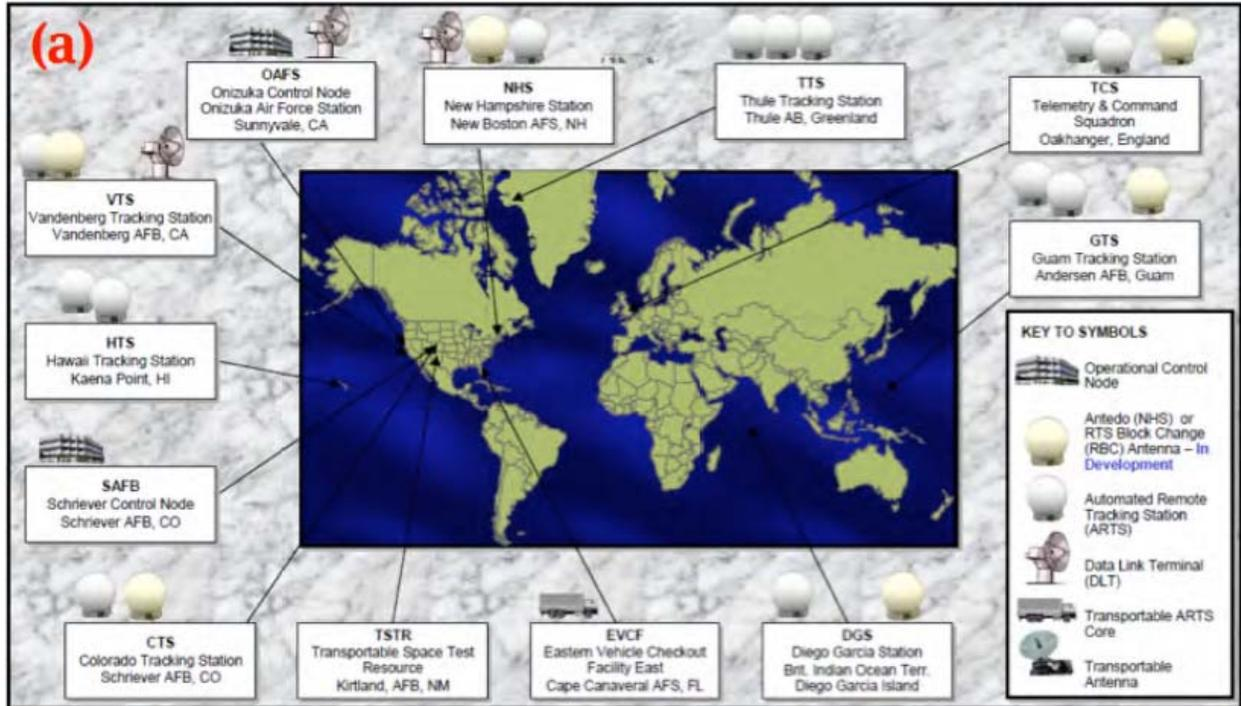
(a) The US Air Force Satellite Control Network (AFSCN) is an example of a conventional hierarchical ground data system setup. Image courtesy of USAF.
