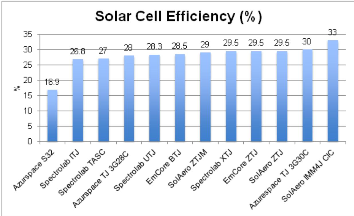
Figure 3.1. Solar Cell Efficiency
