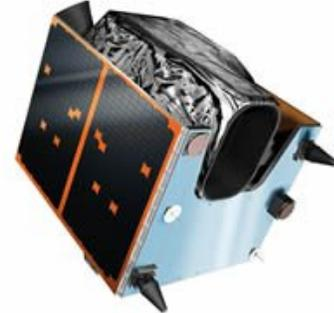
Figure 2.4. The SSTL-150 bus. Image courtesy of Surrey Satellite Technology Ltd. (2015).
