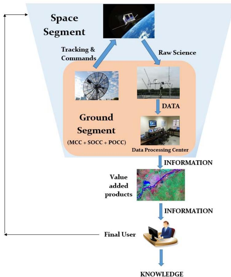
Figure 11.1. Functional relationship between space segment, ground segment and final user in a cubesat mission.
