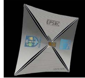
Figure 12.4. AEOLDOS can multiply the average frontal area of a typical cubesat mission almost 100-fold. Image courtesy of Clyde Space (2014).
