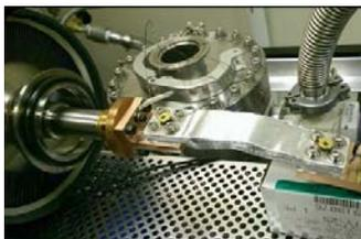
Figure 7.2. Thermal Management Technologies Aluminum thermal strap test. Image courtesy of Thermal Management Technologies (2015).
