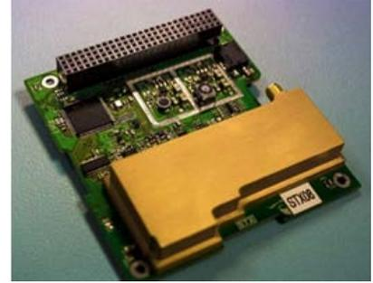
Figure 9.7. Cubesat-compatible S-band transmitter, to be used with either amateur or commercial bands. Image courtesy of Clyde Space.
