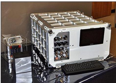
Figure 10.17. NanoRacks Platform 3 image with centrifuge housing. Image courtesy of Nanoracks.
