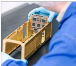
Figure 6.4. C3S 3U CubeSat Structure. Image courtesy of Complex Systems & Small Satellites (2015).
