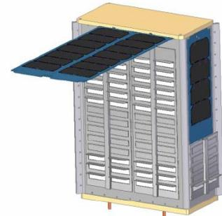
Figure 7.4. Passive Thermal Louver on 6U cubesat Dellinger. Image courtesy of NASA Goddard Space Flight Center (2014).
