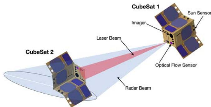
Figure 9.9. Conceptual drawing of laser communication between two cubesats for OCSD mission. Image courtesy of National Aeronautics and Space Administration (2015).
