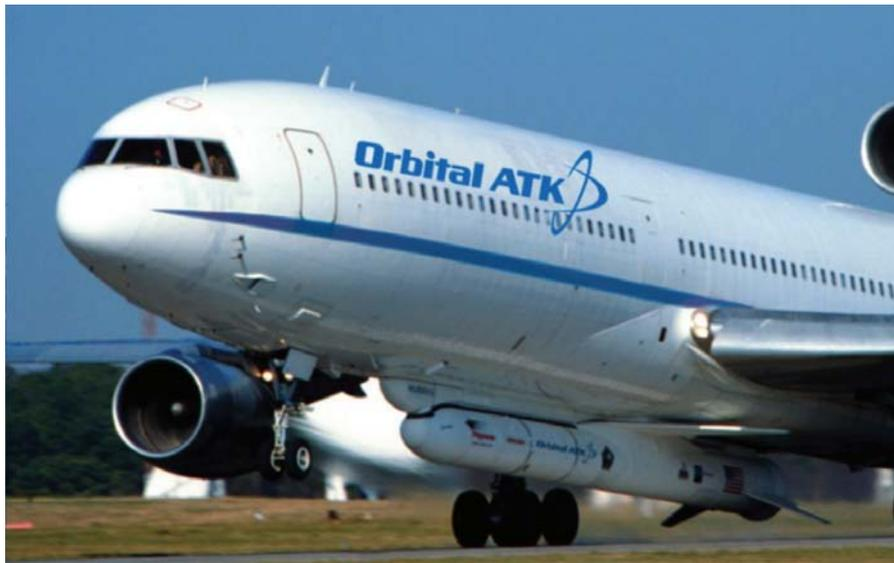
Figure 10.1. Pegasus Launch System, mounted underneath a Lockheed 1011 jet. Image courtesy of Orbital ATK.
