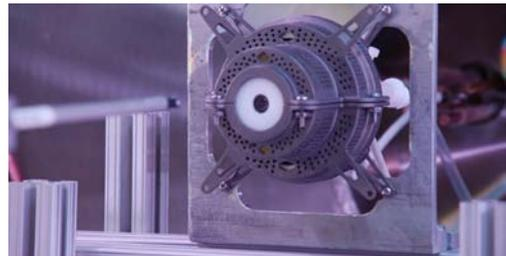
Figure 4.19. Cubesat Ambipolar Thruster (CAT) . Image courtesy of Phase Four LLC.
