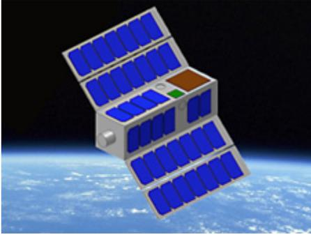
Figure 2.5. The Endeavour bus as used in the CPOD mission. Image courtesy of Tyvak NanoSatellite Systems Inc. (2015a).
