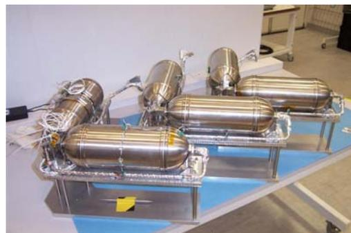
Figure 4.6. SSTL butane propulsion system. Image courtesy of SSTL Gibbon (2010).
