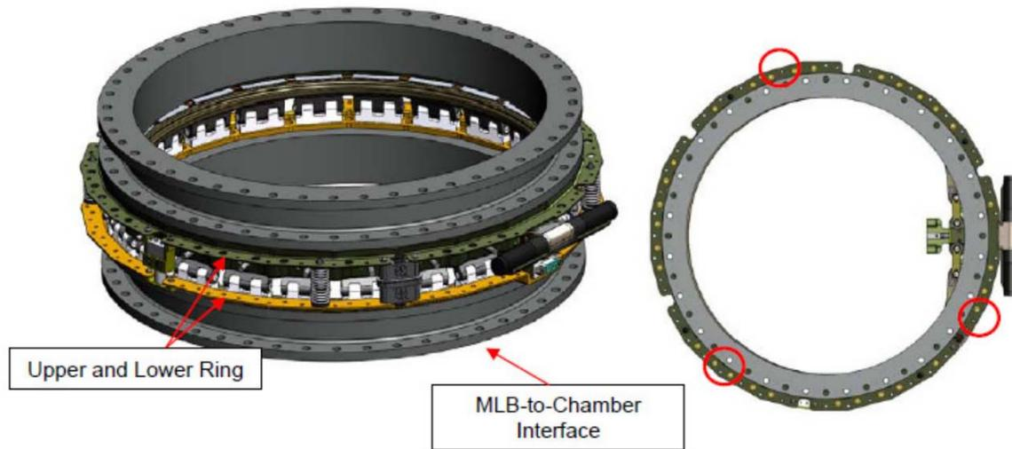
Figure 10.36. MkII Motorized Lightband. Image courtesy of Planetary Systems Corporation.
