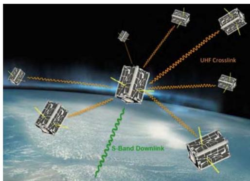
Figure 9.12. Scheme for inter-cubesat communication for EDSN mission. Image courtesy of National Aeronautics and Space Administration (2013b).
