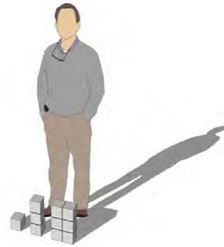
(b) Cubesats with form factors of 1U, 3U, and 6U, respectively. The volume of the 1U base unit is  $100 \times 100 \times 100$  mm.
