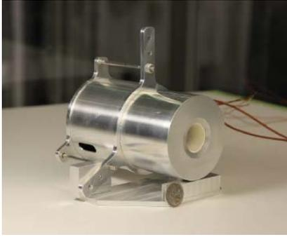
Figure 4.17. Cylindrical Hall Effect Thruster . Image courtesy of UTIAS SFL.
