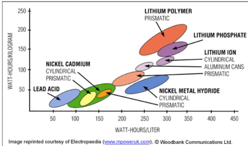
Figure 3.5. The energy densities of various battery types. Image courtesy of Wagner (2006).
