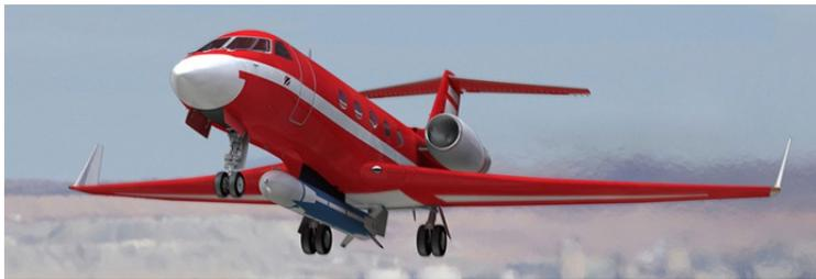
Figure 10.45. GOLauncher System mounted underneath a Gulfstream jet. Image courtesy of Generation Orbit.
