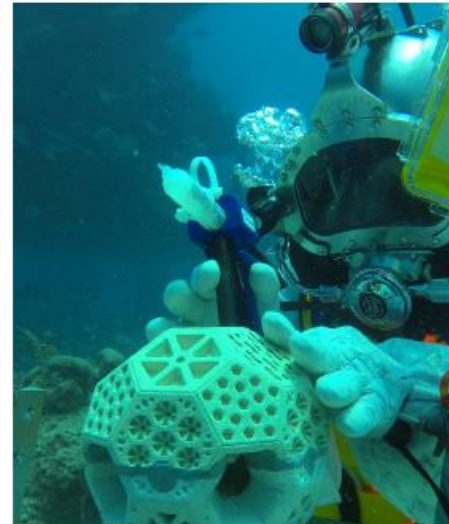
Exploring in-situ repair options on a 3D Printed habitat material
