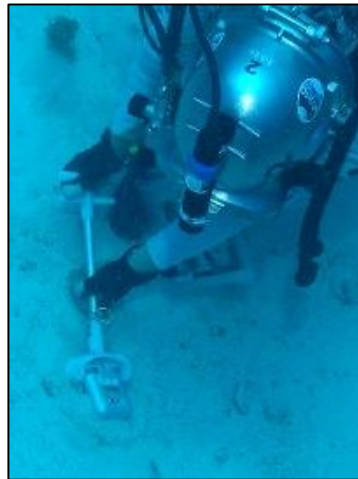
Manual Driver w/ Float/Soil End Effector NEEMO 20
