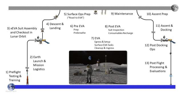
FIGURE 7.2-1: PHASE OF XEVA OPERATIONS FOR LUNAR SURFACE MISSIONS
