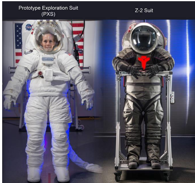
Figure 6. The PXS (left) and Z-2 (right) spacesuits proposed for evaluation during the EVA HHP Benchmarking 2 Study.
