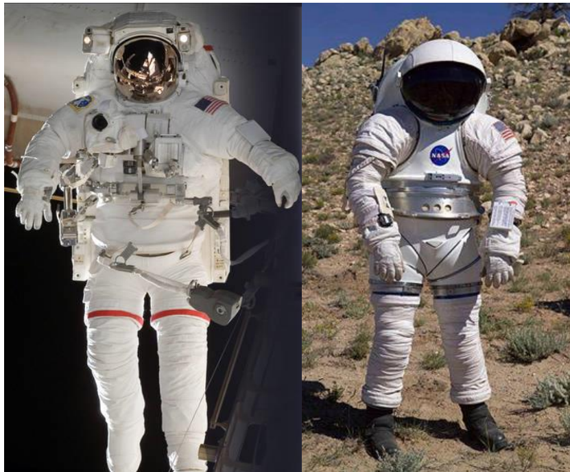
Figure 5. The EMU (left) and Mark III spacesuits planned for evaluation using the EVA HHP Benchmarking methodology.
