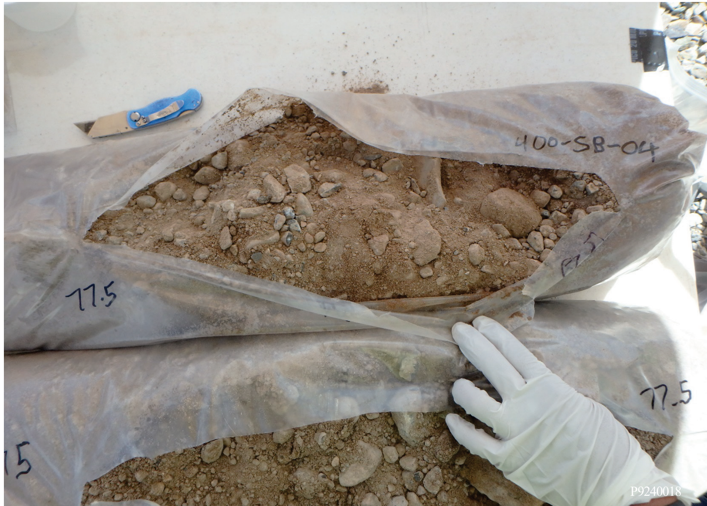
The samples collected in the core barrel during sonic coring were extruded into plastic bags. Each bag was marked with the boring number and the interval from which the sample was collected.
