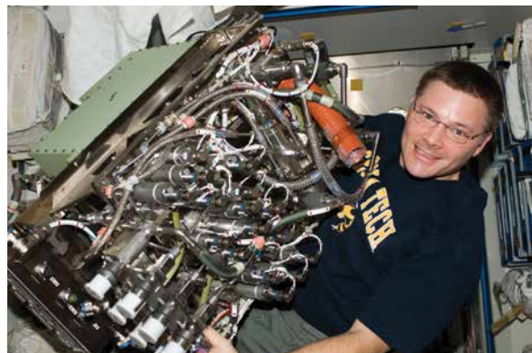
NASA astronaut Douglas H. Wheelock, Expedition 25 commander, is photographed with the Sabatier Assembly - Just prior to installation into Oxygen Generator System rack.
