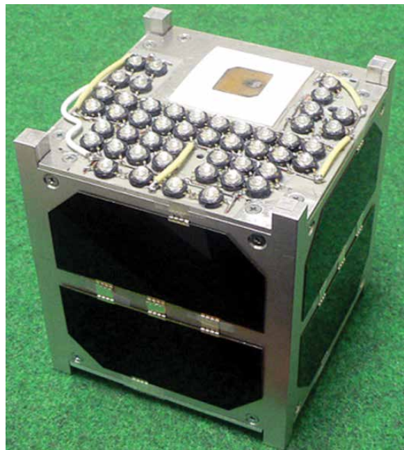
FITSAT, one of the small satellites thrown into orbit by Japanese Experiment Module Robotic Manipulator System.
