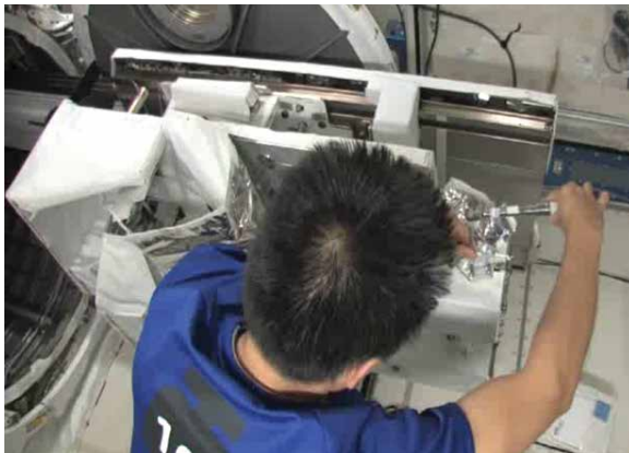
Crew in the International Space Station install a satellite onto the Japanese Experiment Module airlock table.
