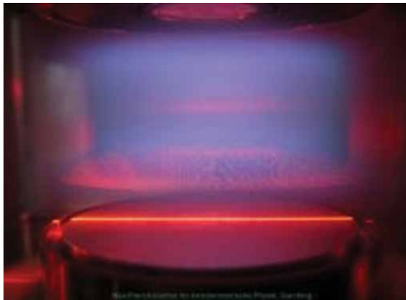
Side view of a plasma crystal in the laboratory. Dust particles are suspended in an argon plasma above a high-frequency electrode (bottom). The horizontal field of view is 2 cm.
