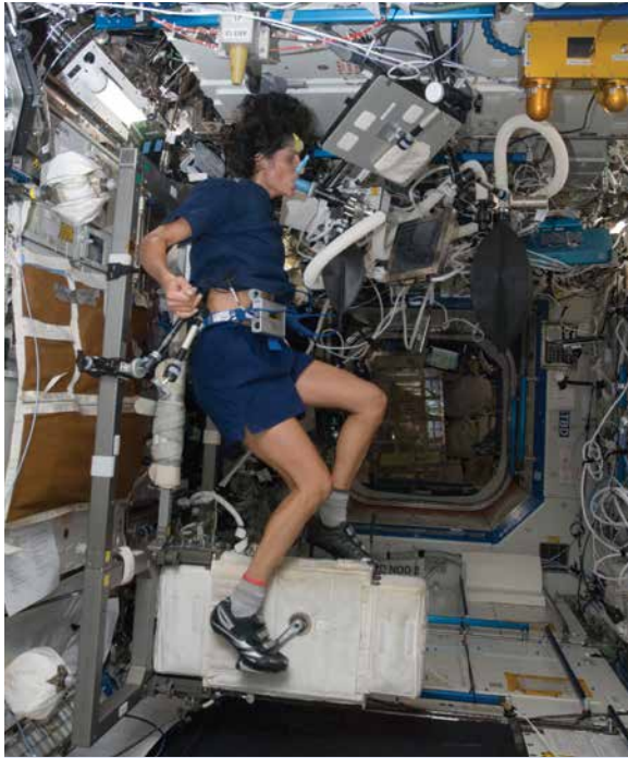
NASA astronaut Sunita Williams uses the Portable Pulmonary Function System whilst on the CEVIS cycle exercise device during a session of the joint Thermolab/EKE/VO2Max experiments in August 2012.
