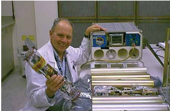
Dr. Dennis Morrison poses with the Microencapsulation Electrostatic Processing System flight hardware that was used on the International Space Station to produce microcapsules for cancer treatment delivery.
