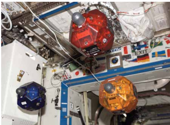
The three Synchronized Position Hold, Engage, Reorient Experimental Satellites (SPHERES) on the space station are considered facilities. Two are used for Zero Robotics.
