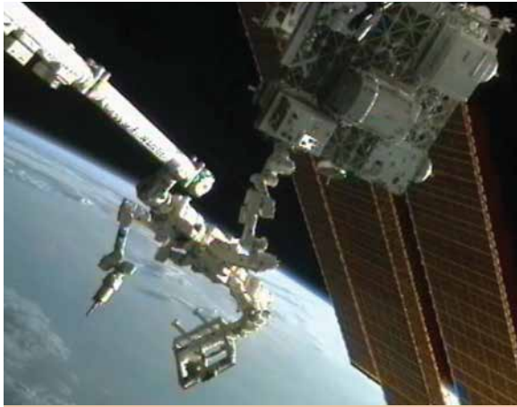
The Robotic Refueling Mission investigation (center, on platform) uses Canadarm2, the International Space Station's robot arm, and the Canadian Dextre robot (right) to demonstrate satellite-servicing tasks.
