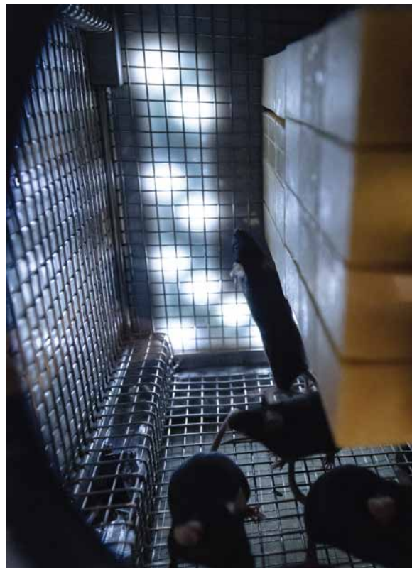
A view inside of the NASA Rodent Research facility, self-contained habitat that provides its occupants living space, food, water, ventilation, and lighting. Cabin air is exchanged with the facility, creating a slight negative pressure inside the cage to pull animal waste into a collection filter.
