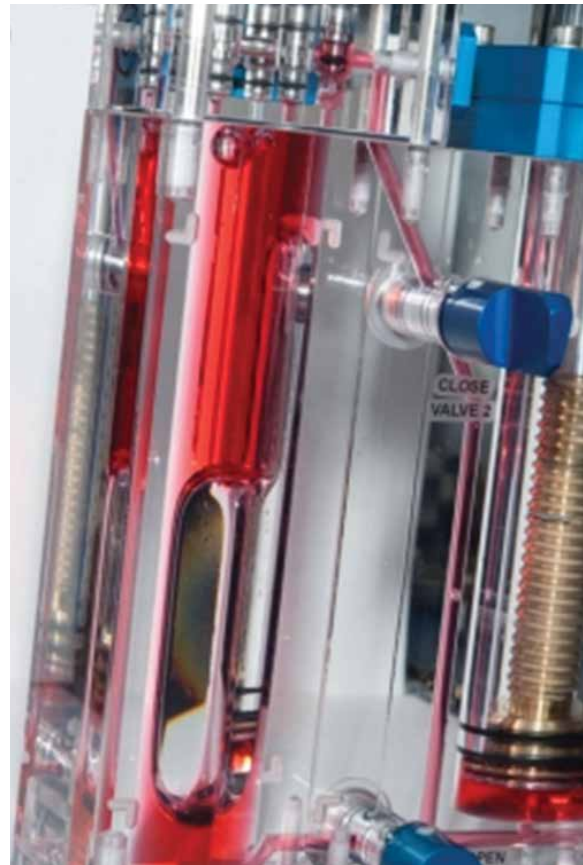
A view of Capillary Flow Experiment - 2 Interior Corner Flow 3 vessels set up during an experiment aboard the International Space Station. This study looks at capillary flow in interior corners.
