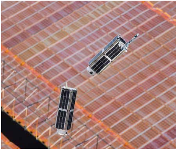
Two Planet Labs "Dove" CubeSats immediately after being deployed from the ISS.
