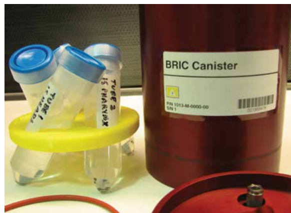
Flatworms being prepared for loading into the Biological Research In Canisters hardware.
