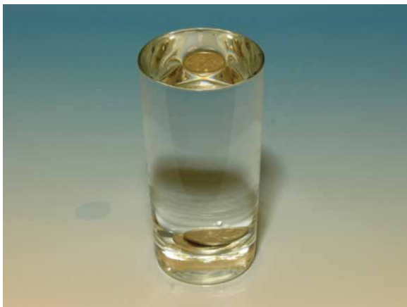
A coin floats on the surface of the water because of surface tension. Image credit: JAXA
