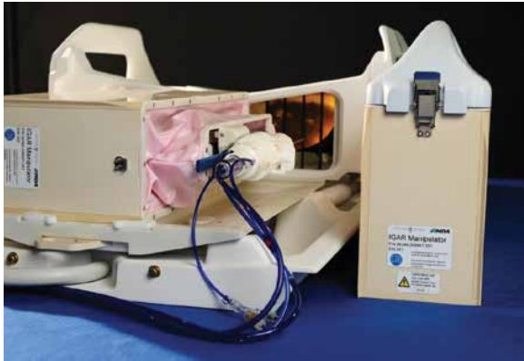
IGAR manipulator and full breast intervention platform mounted on the patient support structure with a biopsy tool attached.
