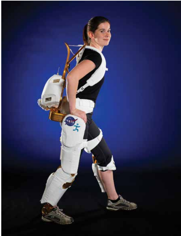
NASA Project Engineer Shelley Rea demonstrates the X1 Robotic Exoskeleton, which could improve the mobility and strength of astronauts and paraplegics.
