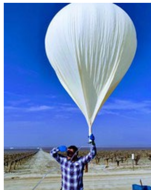
Balloon flights conducted by Black Sky Aerospace in early 2019 enabled preliminary testing of The Aerospace Corporation's method for Rapid Calibration of Space Solar Cells. Credit: Colin Mann/The Aerospace Corporation
