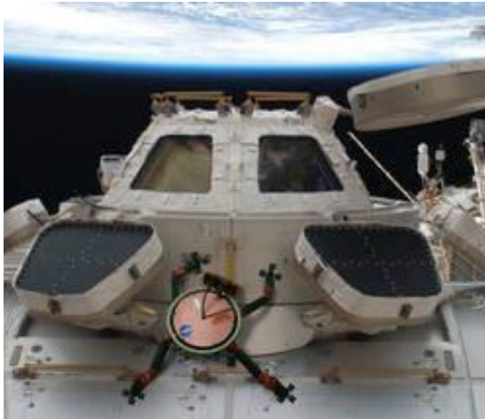
An artist's concept shows how a future robot called LEMUR (Limbed Excursion Mechanical Utility Robot) could inspect and maintain installations on the ISS, sticking to the outside using the gecko-inspired technology. Credit: NASA/JPL-Caltech
