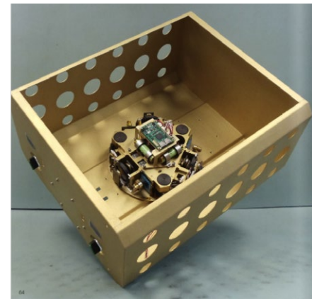
The Vibration Isolation Platform technology is shown here, inside a mid-deck locker insert.
