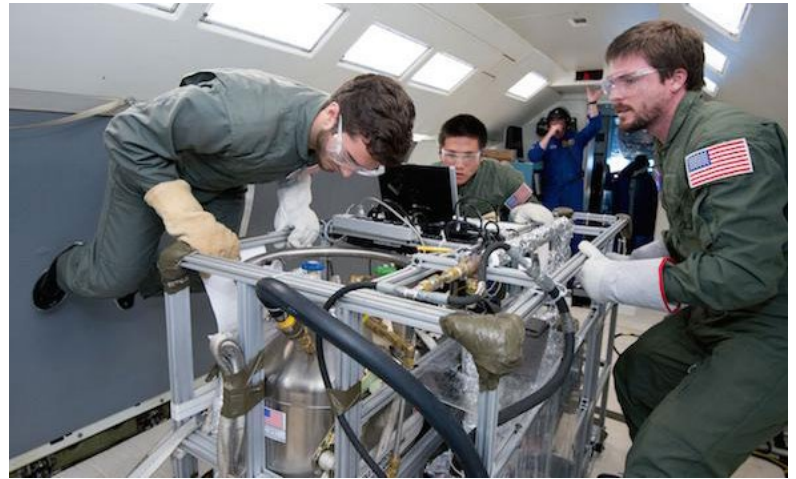
Cryogenic propellant chill-down experiments from the University of Florida have accumulated data over multiple parabolic flight campaigns. Others flew for the first time on ZERO-G's recent flights. NASA photo.
