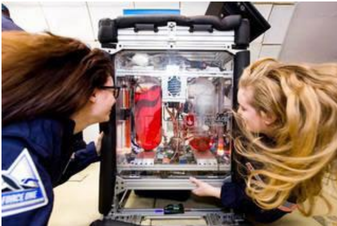
Carthage College students and Microgravity Propellant Gauging team members Taylor Peterson and Celestine Ananda observe tanks during a parabolic flight in November 2018. The suborbital payload is smaller and designed to test how the gauging technology will work with settled, non-sloshing liquids. Credit: Steve Boxall/Zero Gravity Corporation
