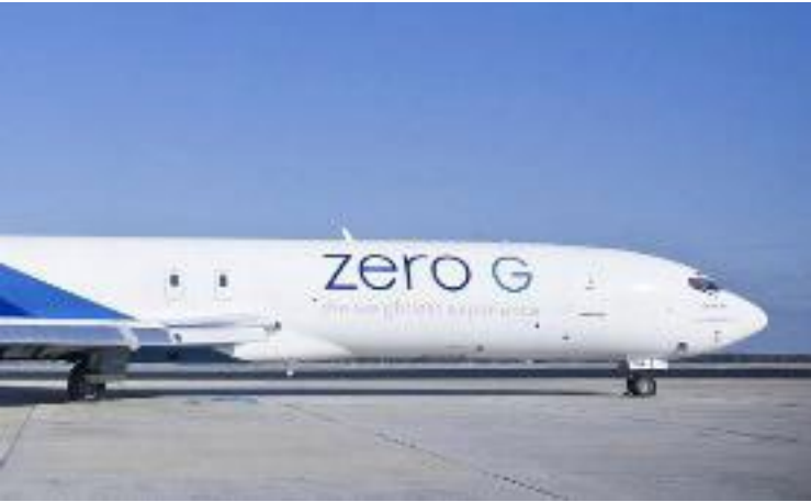
ZERO-G's G-FORCE ONE aircraft is a Boeing 727-200F modified for reduced gravity environments.
