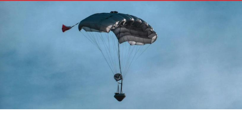
The SpaceWorks RED-4U capsule in flight after being released from a Near Space Corporation high-altitude balloon at 103,000 feet. The parafoil guiding the capsule's descent was developed by Earthly Dynamics Corporation and Aerial Delivery Solutions. Credit: SpaceWorks Enterprises, Inc.
