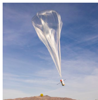
In a flight test over Lemitar, New Mexico, a balloon from Raven Aerostar carries technology from Sandia National Laboratory and NASA's Jet Propulsion Laboratory that could be used to aid seismology studies on Venus and other planets. Credit: Sandia National Laboratory
