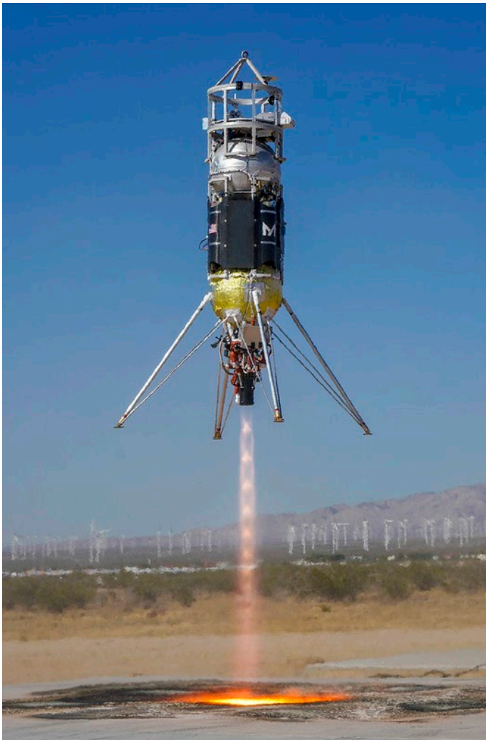
Masten Space Systems' Xodiac vertical takeoff and vertical landing system lifts off the desert floor at Mojave Air and Space Port in California. Credits: Masten Space Systems/Matt Kuhns
