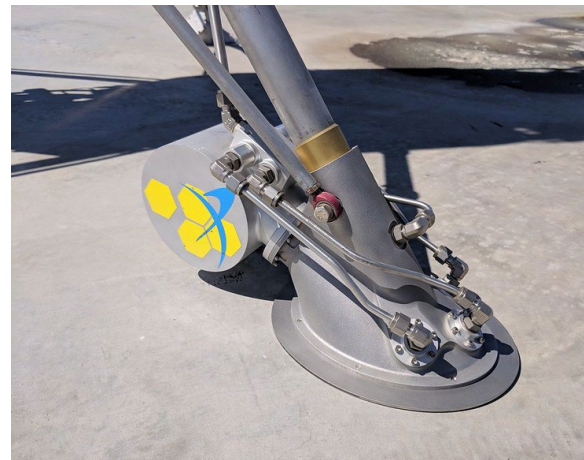
PlanetVac uses suction to lift regolith into a canister for separation and storage. Credit: Honeybee Robotics
