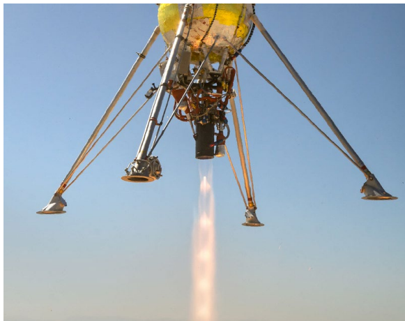
PlanetVac is shown attached to the leg of Masten's Xodiac vehicle. Credit: Honeybee Robotics
