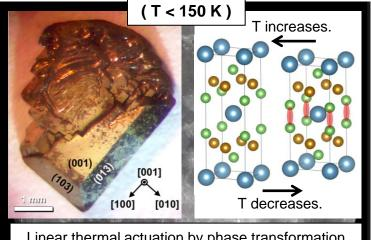
Linear thermal actuation by phase transformation
