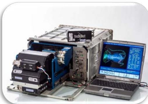
Full densitometer system featured above with a single laptop to drive the system. The entire system easily fits on a small tabletop.
