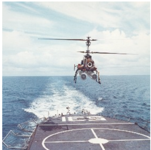
The Gyrodyne QH-50 takes off of a U.S. Navy assault ship < https://www.vtol.org/uavpaper/NavyUAV.htm >.
