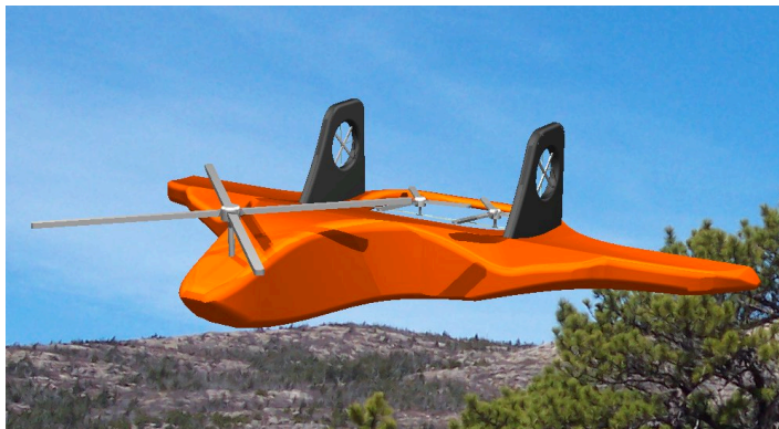
Fig. 9 Showing vertical flight with the rotors facing upwards
