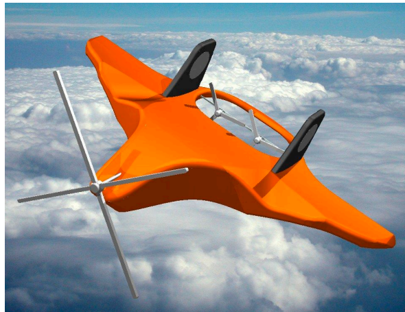
Fig. 6 Showing horizontal flight with the rotors facing forwards
