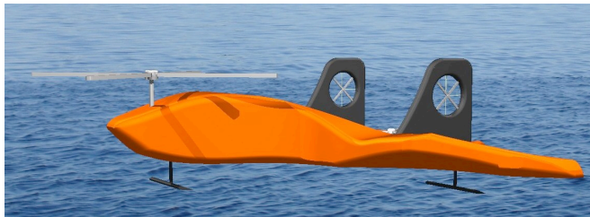
Fig. 3.1 Showing extended hydrofoils
