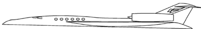
Figure 3: An example of structural configuration of an aircraft that incorporates design elements to shape the sonic boom (based on an illustration in Henne's patent 15 )
