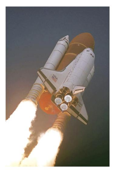
At liftoff, the two **Solid Rocket Boosters** consume 11,000 pounds of fuel per second. That's two million times the rate at which fuel is burned by the average family car.
