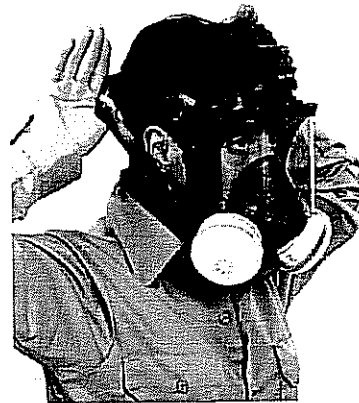
FIGURE 6 Placing the Facepiece on Your Head
