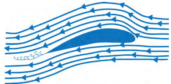
Fig. 3 Air approaching and passing over the surface.
