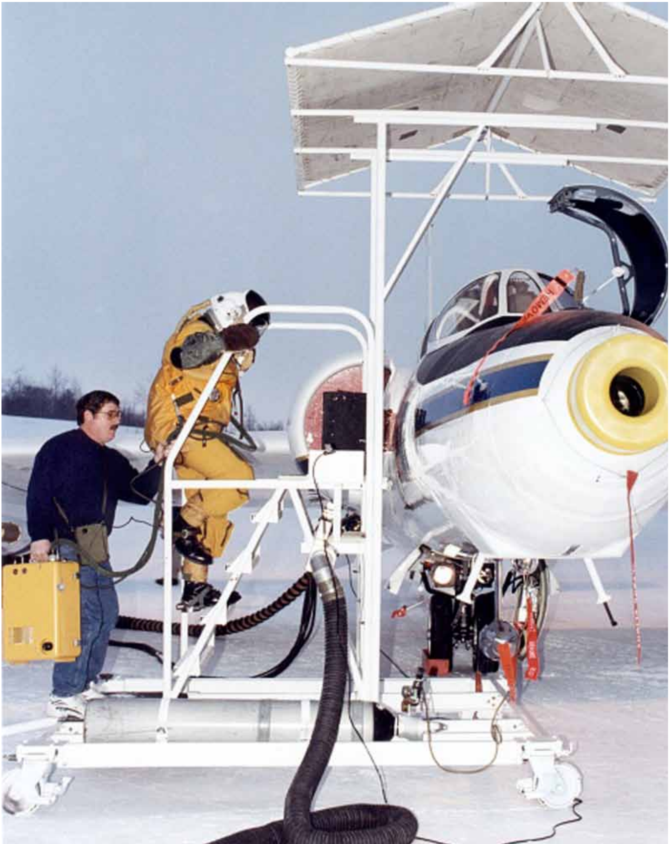
A life-support technician assists a pressure-suited pilot into the cockpit of NASA's ER-2 earth resources aircraft. (Image Credit: NASA, http://www.dfrc.nasa.gov/Gallery/Photo/ER-2/Small/EC00-0037-27.jpg )
