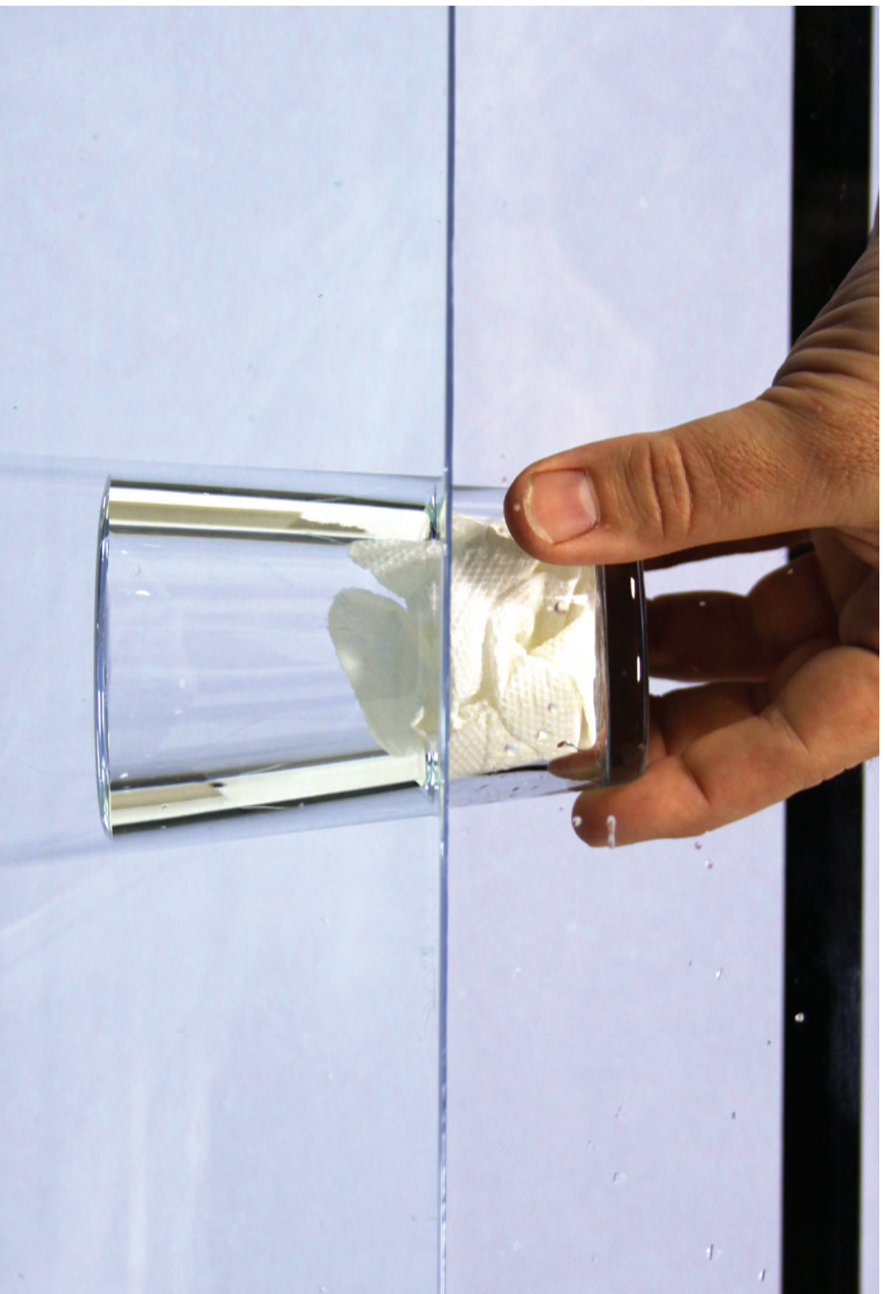
Img. 5 Air in the glass prevents the water from entering
