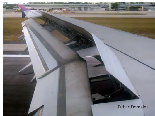
Img. 1 Ground spoilers on an Airbus 320 aircraft
