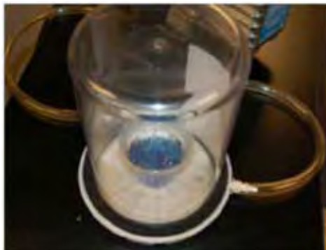
Water boiling in a vacuum.
