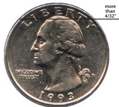
Fig. 7 Quarter (head) tread measurement
