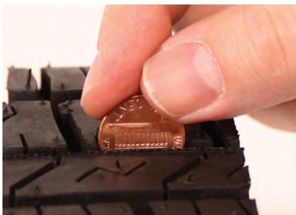
Fig. 8 Penny (tails) tread measurement
