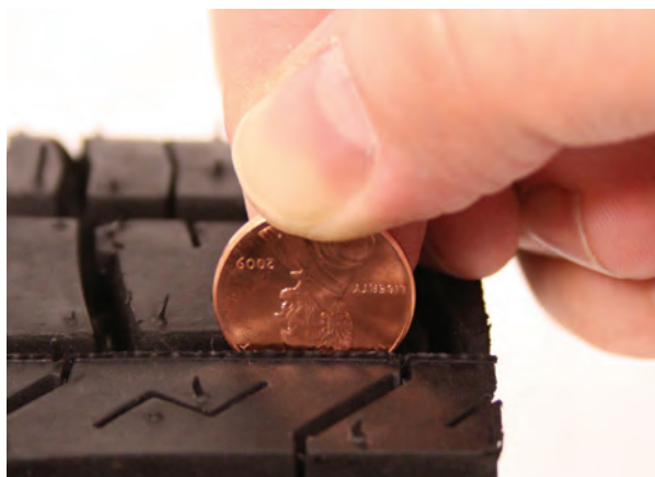
Fig. 6 Penny (head) tread measurement
