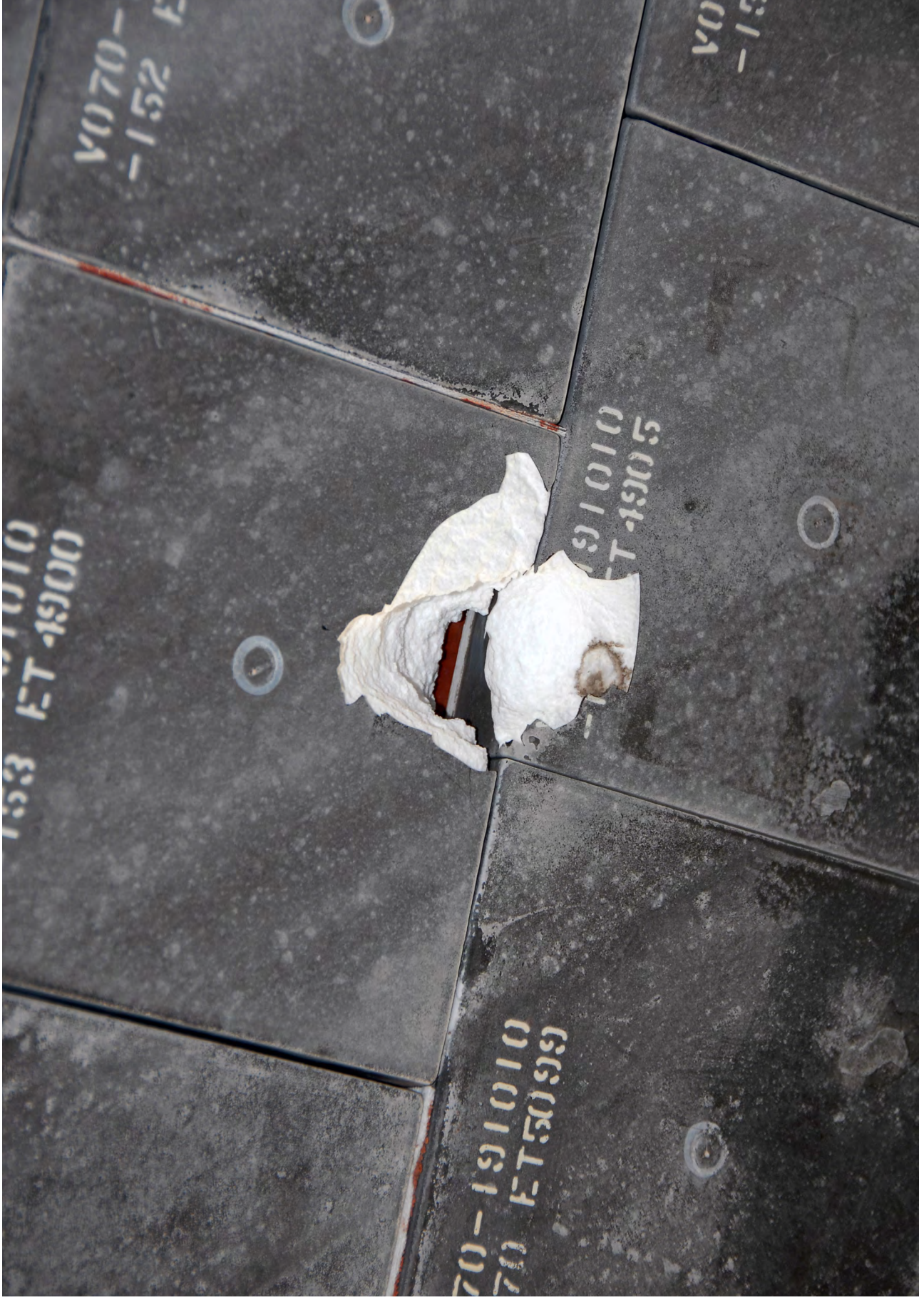
Img. 4 Shuttle tile showing signs of damage.
