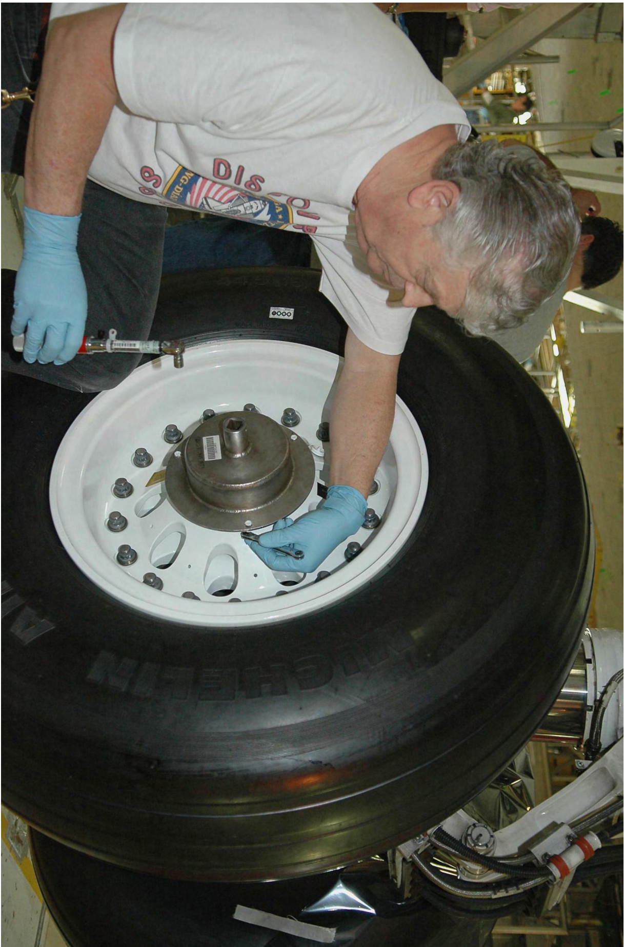
Img. 3 Installing a main shuttle tire
