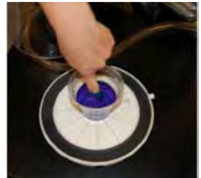
Testing water temperature immediately after the water leaves the vacuum environment.
