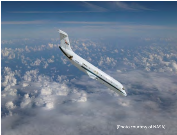
Img. 4 "NASA 932" Weightless Wonder VI, Vomit Comet Completing a Parabola
