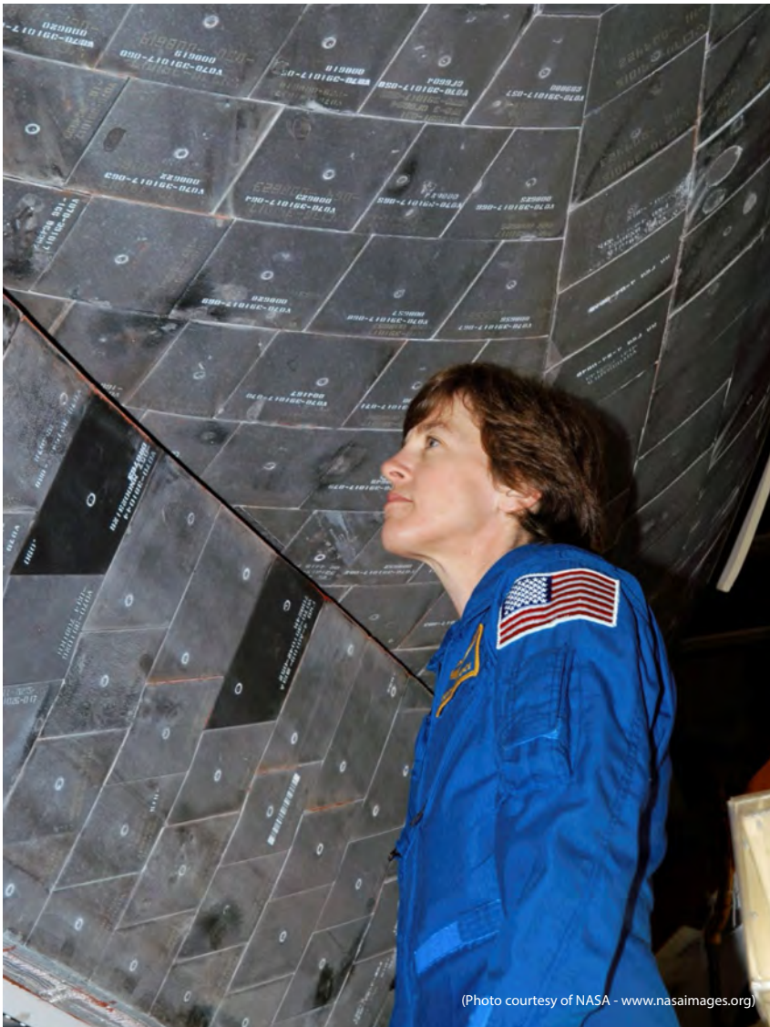
Img 5. A close-up of the tile numbering system.
