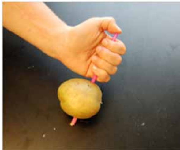
When the end of the straw is blocked, pressure increases inside the straw as it is pushed into the potato, thus increasing the rigidity of the straw and preventing buckling.
