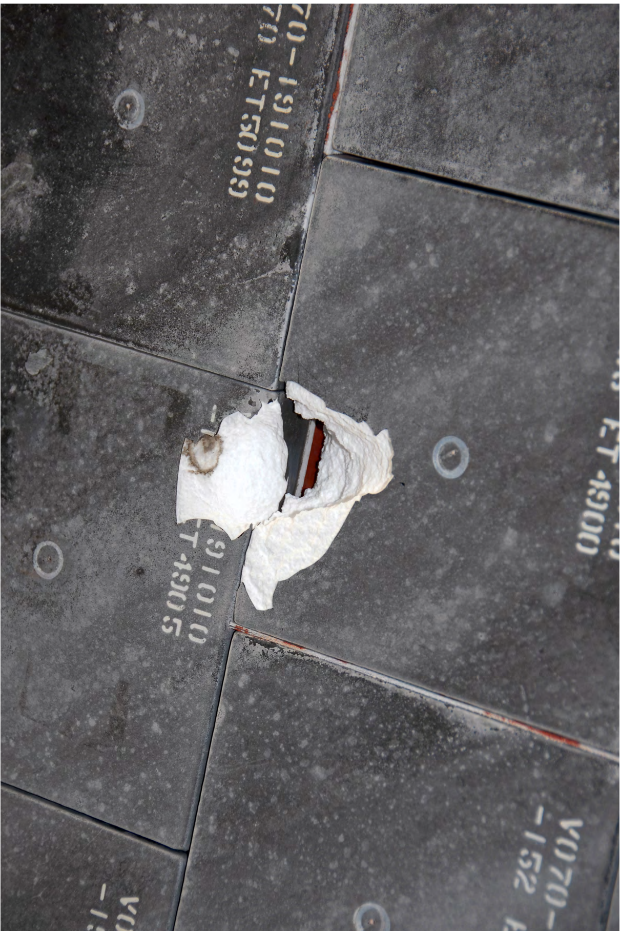
Img. 4 A damaged tile from Space Shuttle Endeavor. The tile was damaged on Mission STS-118 when a piece of foam from the external tank broke off during launch.
