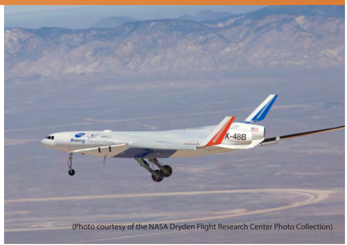
X-48B Blended wing body during its first flight on July 20, 2007
