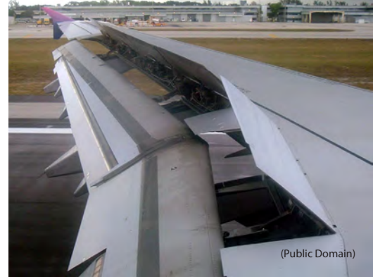
Img. 1 Ground spoilers on an Airbus 320 aircraft
