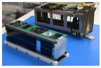
CSSWE was developed and built by the University of Colorado and funded by the National Science Foundation to perform orbital onboard space weather measurements. The CubeSat will measure the directional differential flux of Solar Energetic Protons (SEPs) and Earth's radiation belt electrons to support the Radiation Belt Storm Probe mission and help to understand the relationship between SEPs, flares and coronal mass ejections.
