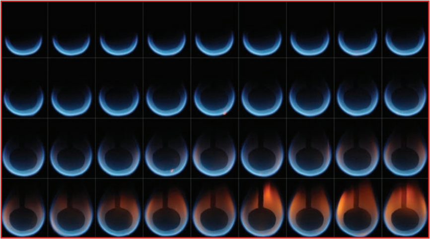
Figure 11. Flame sequence of a burning 2-cm diameter acrylic sphere at 17 percent oxygen and 12 cm/s flow from the Burning and Suppression of Solids experiment. The images are about 1.5 sec. apart. With the reduction in oxygen from 21 percent (air) to 17 percent, the flame stays bluer much longer (soot formation is delayed) facilitating comparison with model. The high-resolution images allow model comparison of flame growth rate, flame-to-fuel distance, and the solid regression rate.
