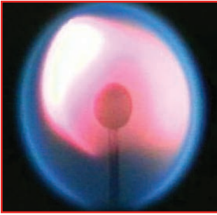
Figure 6. Image of a spherical diffusion flame on a porous burner (which is also visible) at the end of a test conducted in NASA's 2.2-second Drop Tower. The gas from the burner was 1.51 mg/s of 100 percent ethylene issuing into air at atmospheric pressure. (Image credit: NASA, ACME project, Flame Design experiment)
