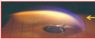
Figure 9. Flame spreading preferentially upstream in slow convective flow. (Image credit: NASA, Radiative Ignition and Transition to Spread Investigation experiment)
