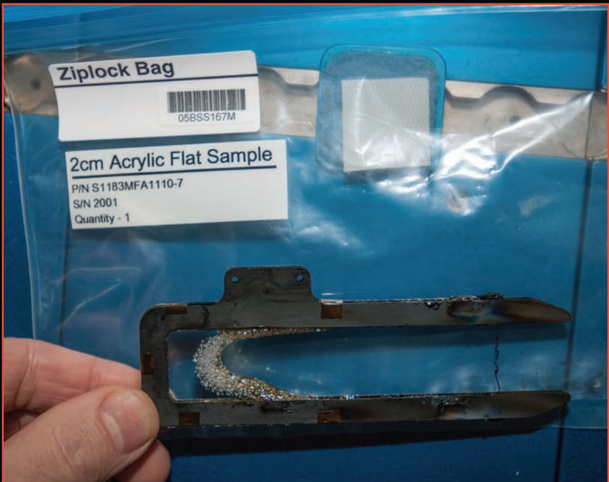
Astronaut holding a sample holder with a burned and bubbled acrylic sheet from the Burning and Suppression of Solids (BASS) experiment conducted in the Microgravity Science Glovebox on the International Space Station. (Image credit: NASA, BASS experiment)
