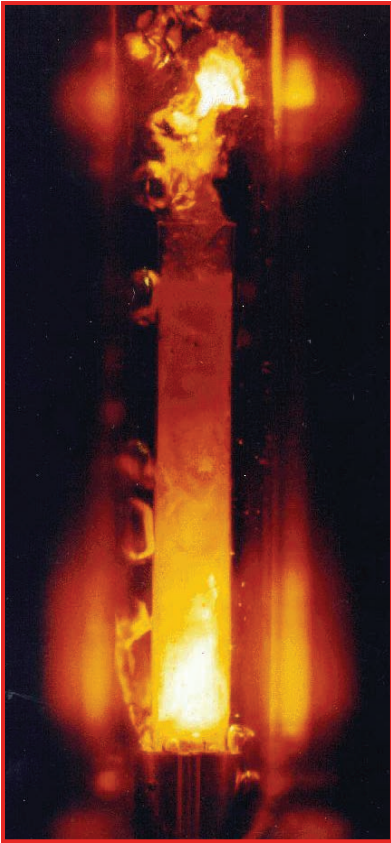
Figure 20. Hydrothermal flame existing in a super-critical core region surrounded by a sub-critical annular region (Wellig, B., Swiss Federal Institute of Technology, Zurich).
