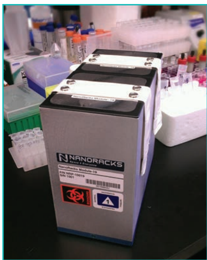
NanoRacks-Protein Crystal Growth-1 (NanoRacks-PCG-1) is a proprietary protein crystal growth housed inside NanoRacks Module-19. Image is courtesy of Carl W. Camuthers, Jr.
