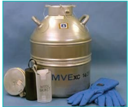
NASA's Kennedy Space Center (KSC) Gaseous Nitrogen Freezer with lid removed. (Image is courtesy of KSC.)
