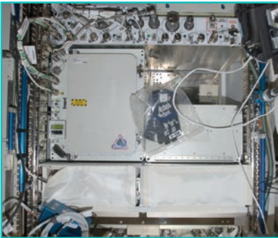
View of the general Laboratory Active Cryogenic ISS Experiment Refrigerator within EXPedite the PROcessing of Experiments to Space Station Rack 6 in the U.S. Destiny Laboratory during Expedition 18.
