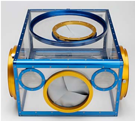
Figure 7. The AAU provides containment during animal access and transfer between the Transporter, Rodent Habitat, and the Microgravity Science Glovebox. The bottom of the unit is open to provide access to doors in the Transporter and Habitat hardware that are opened after the Animal Access Unit is attached.
