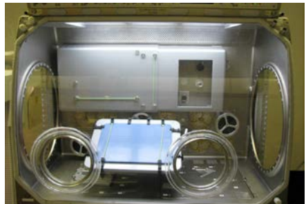
Figure 11. The Microgravity Science Glovebox is a sealed workspace with built-in gloves (not shown) that safely contains fluids, flames, particulates, and fumes, and allows handling of small equipment.
